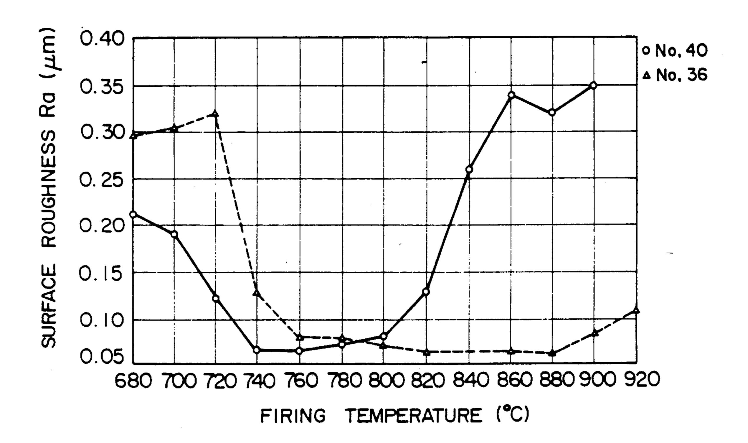
GLASS CERAMIC FOR COATING METAL SUBSTRATE
