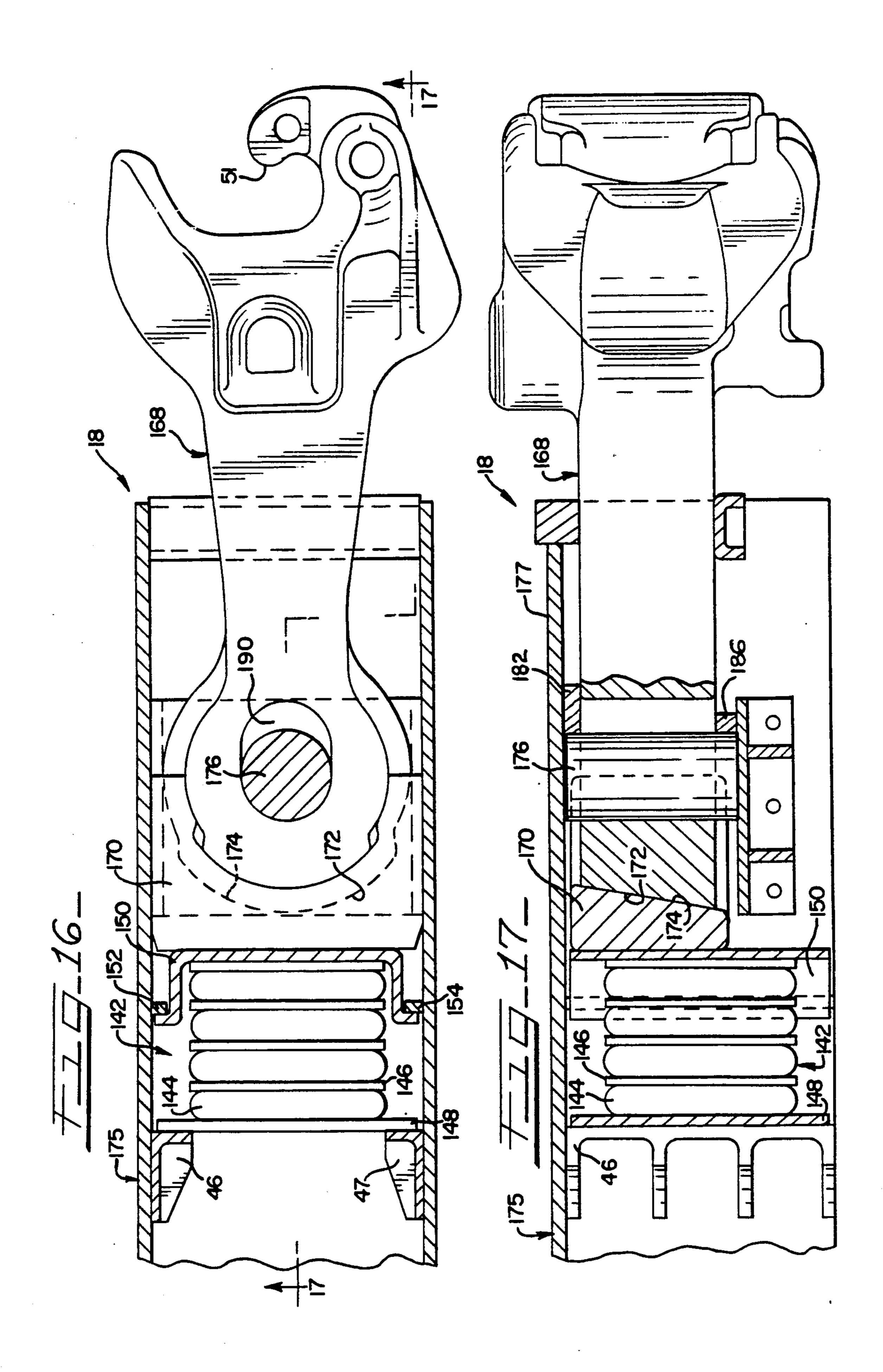
restraining the butt end of the coupler member in a lateral and longitudinal position within the center sill.
