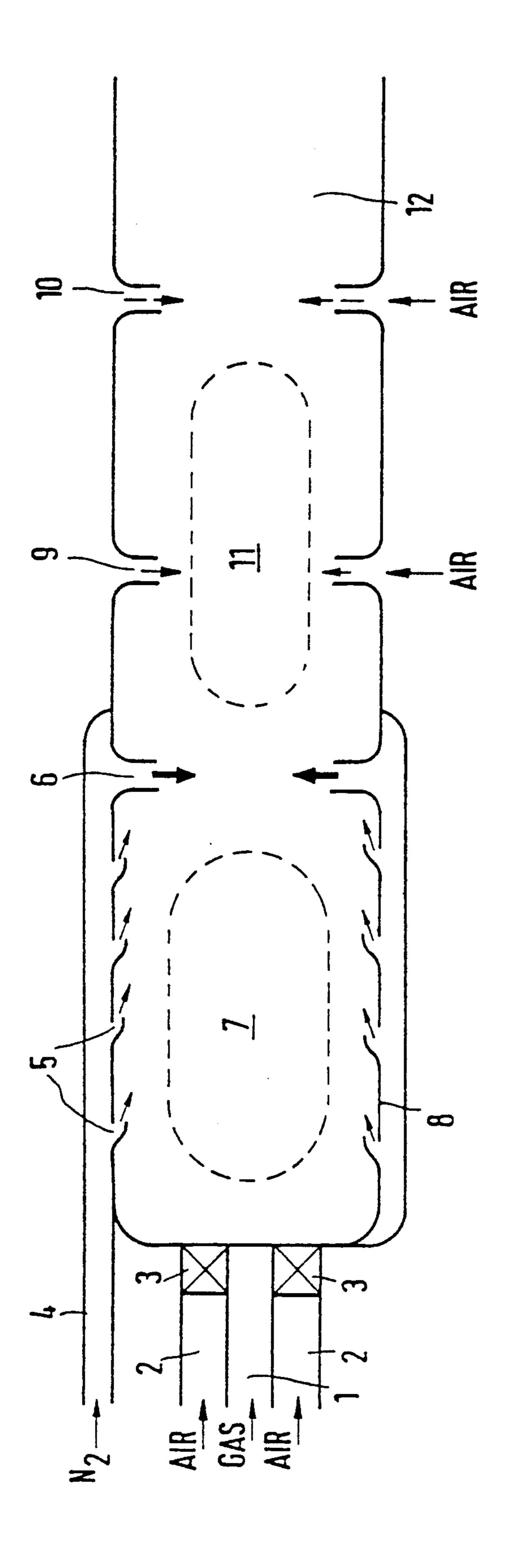
MUTI-STAGE COMBUSTION CHAMBER FOR COMBUSTION OF NITROGEN-CONTAINING GAS WITH REDUCED NO<sub>x</sub> EMISSIONS, AND METHOD FOR ITS OPERATION
