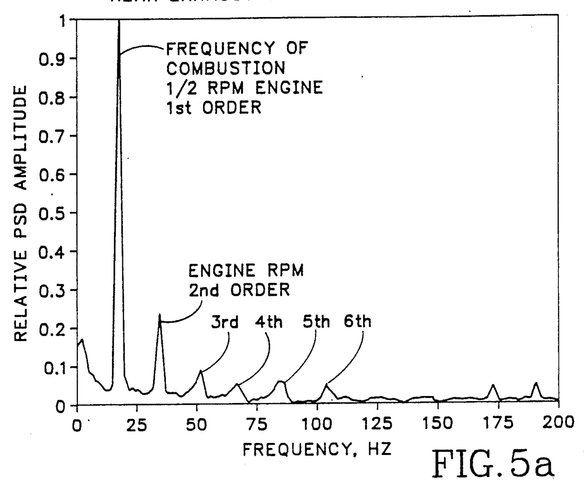
GM ENGINE: KNOCK CONDITIONS NEAR EXHAUST VALVE: 1840 RPM=30.7 HZ
