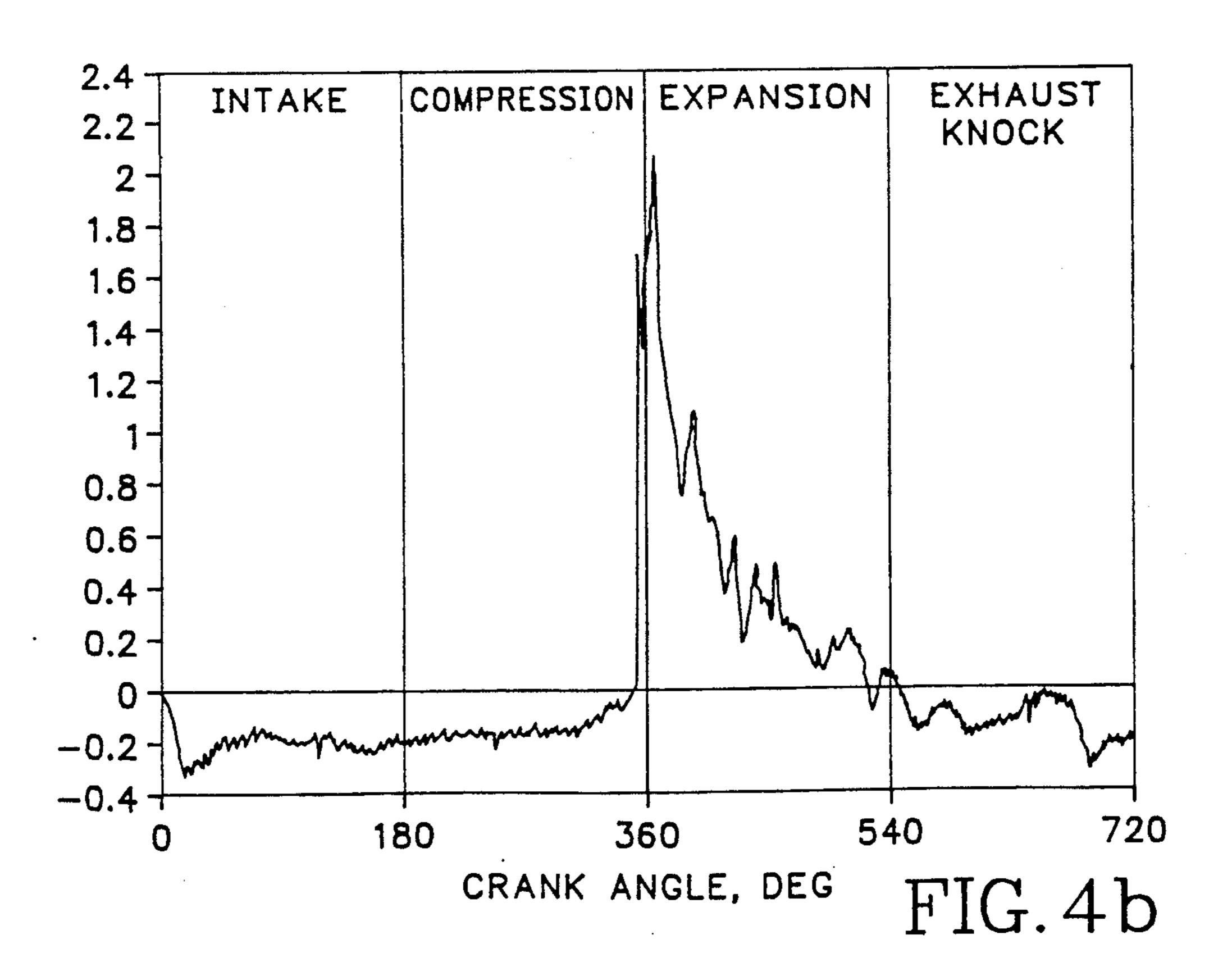
GM ENGINE: NORMAL CONDITIONS NEAR EXHAUST VALVE: 2090 RPM=34.8 HZ
