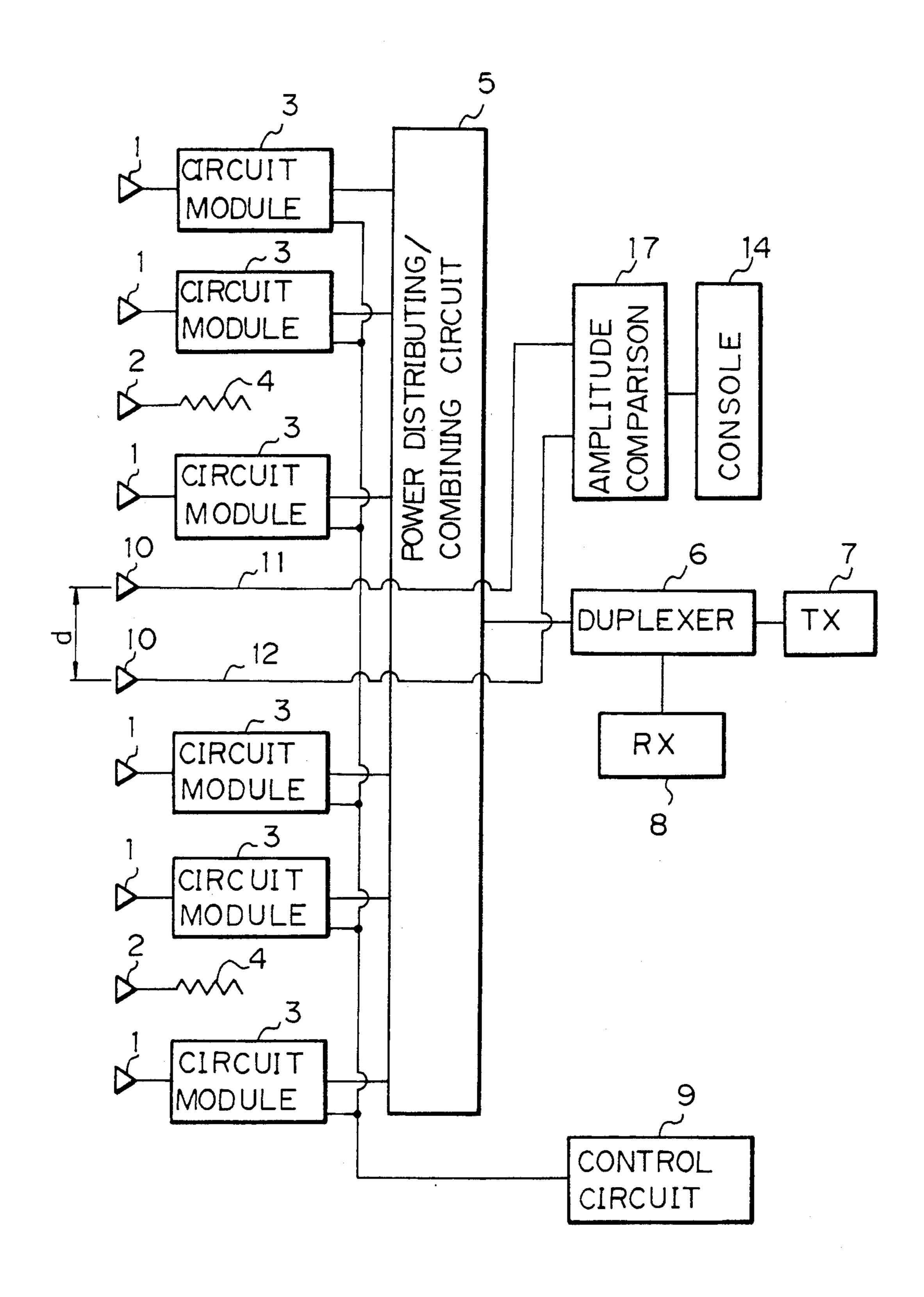
ARRAY ANTENNA SYSTEM WITH DIRECTION
