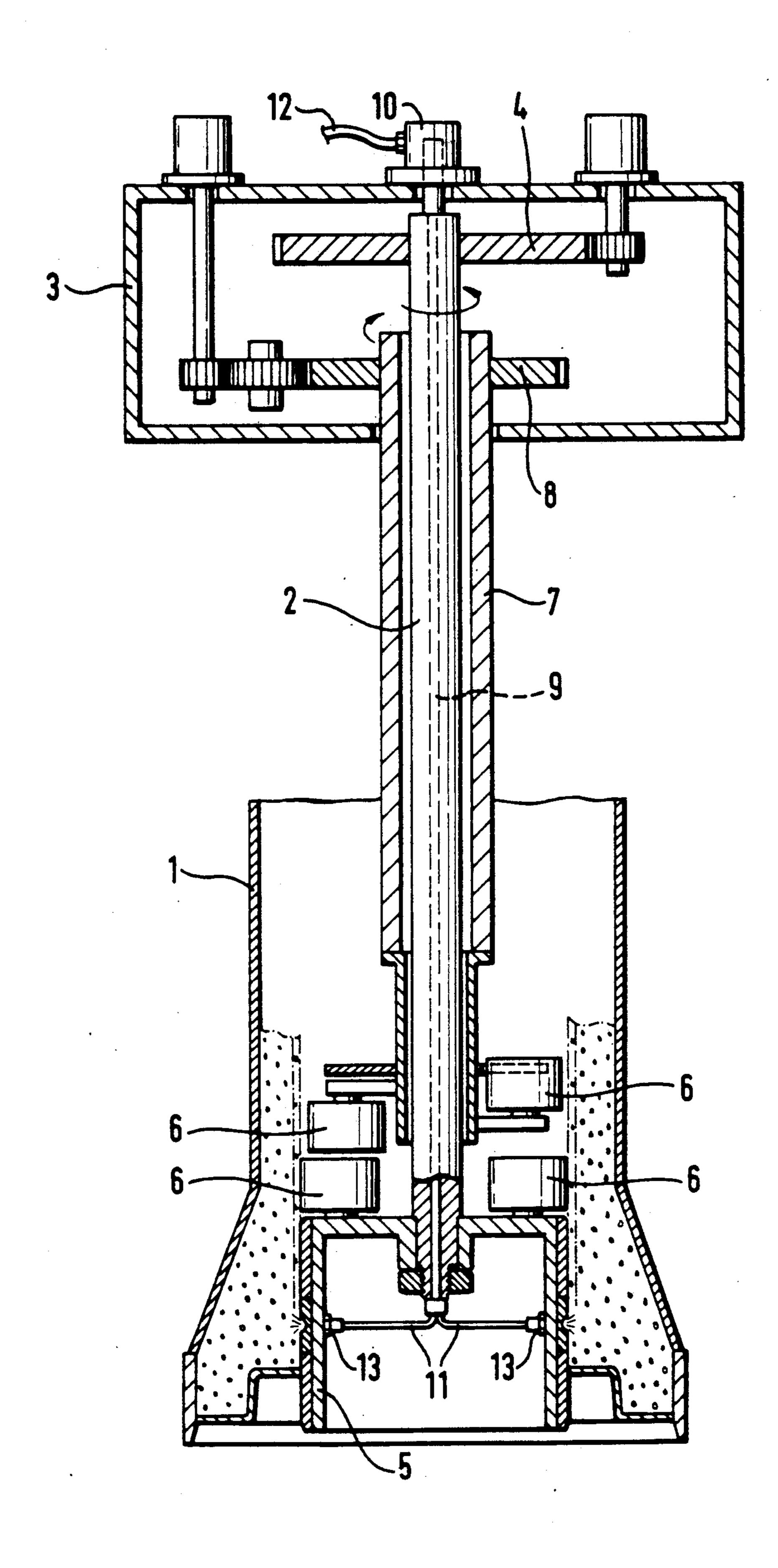
METHOD FOR THE PRODUCTION OF CONCRETE PIPES
