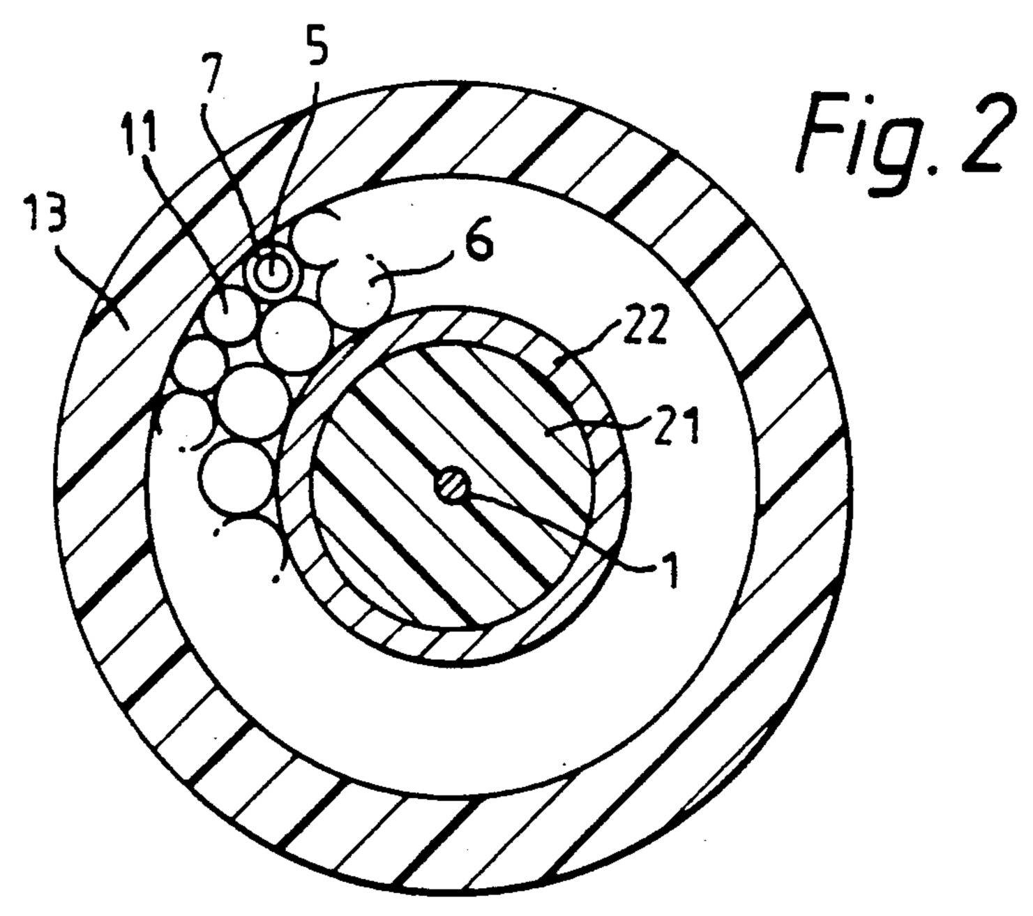
counts, so it is desirable to have the freedom to vary the number of tubes replacing strength members in a layer, without affecting torsional performance significantly.
