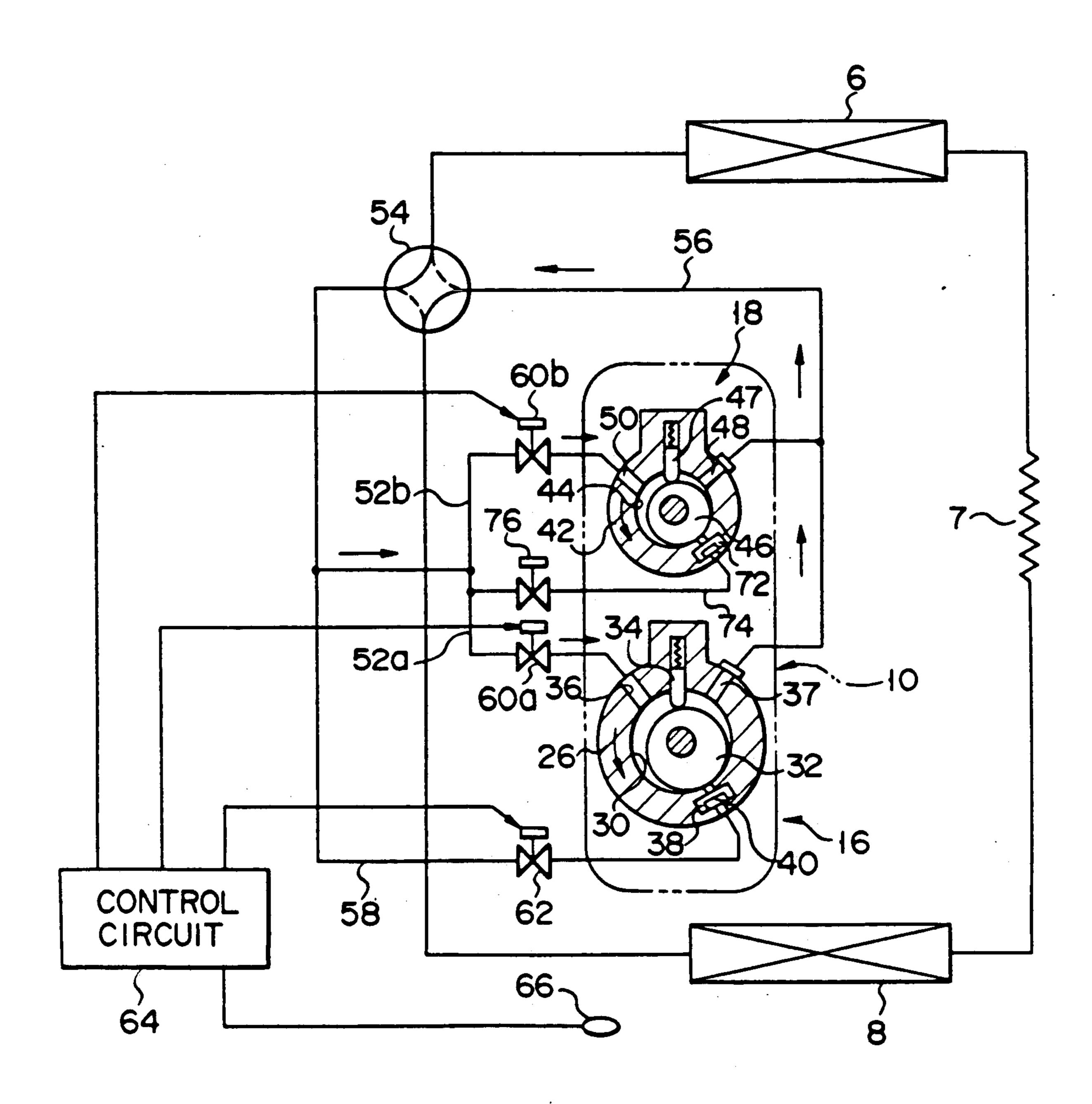
rotary compressor whose capacity can be variously changed without using an inverter circuit.
