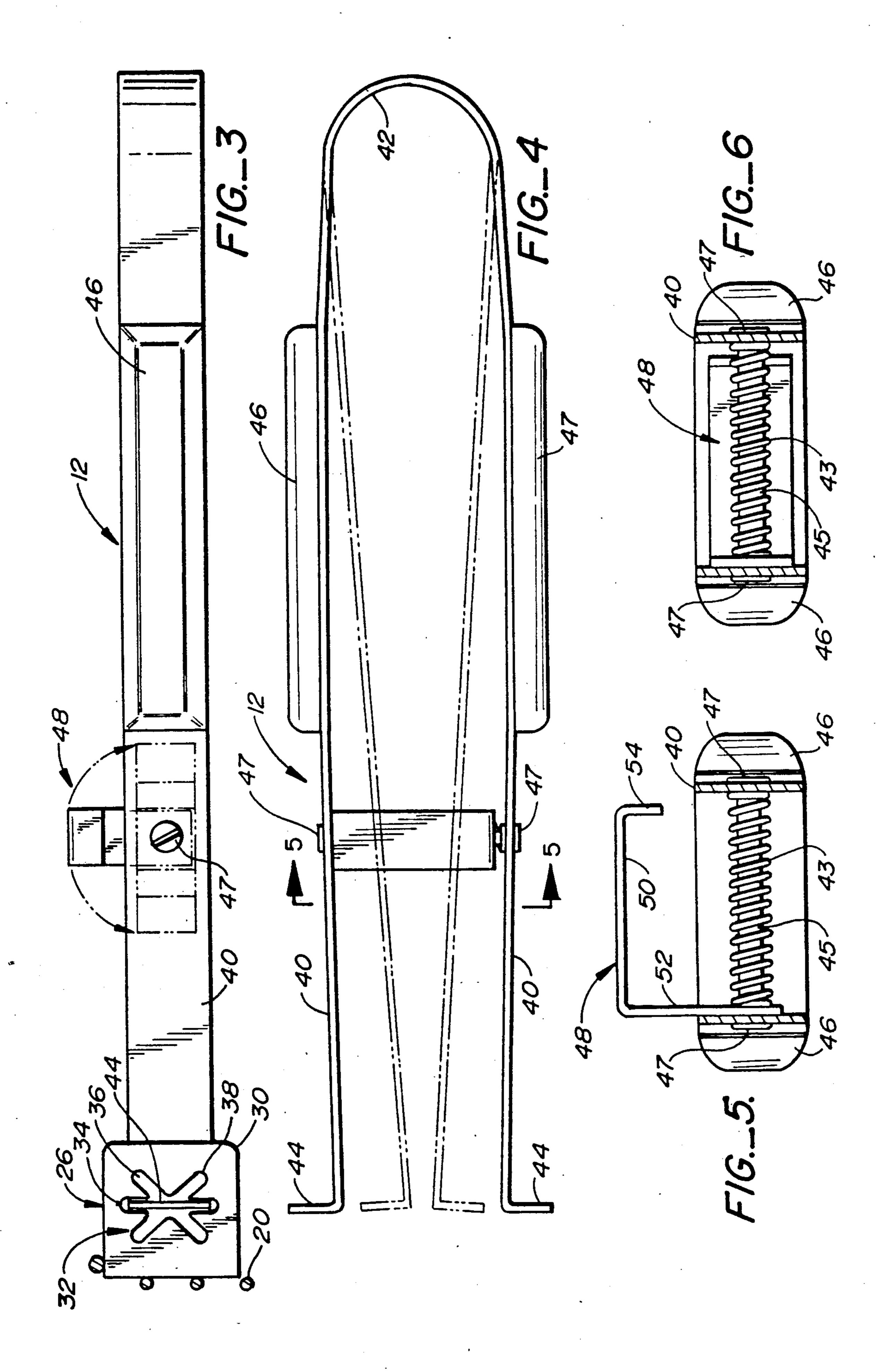
the tong arms thereby providing three different angular positions for the handle relative to the basket.
