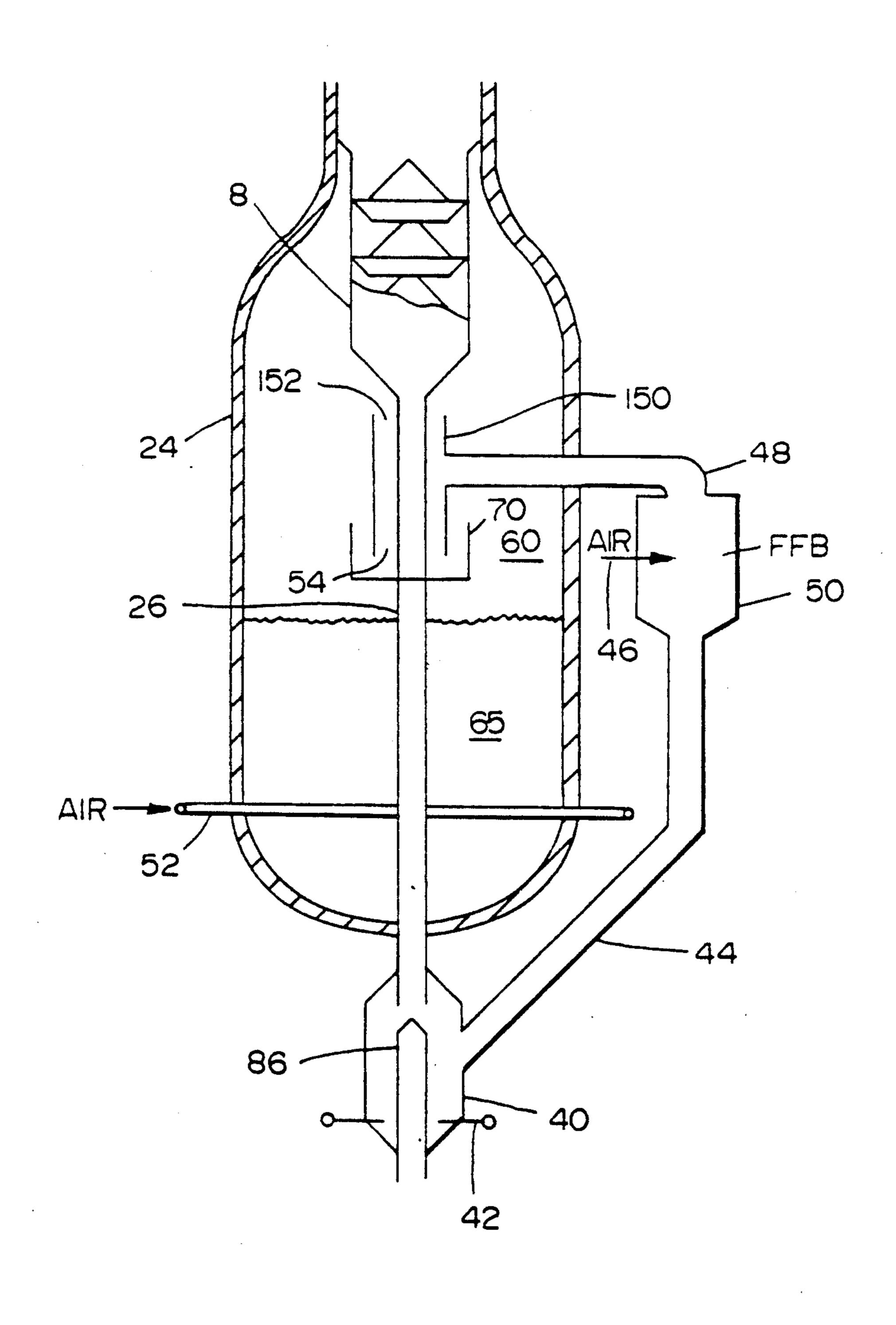
PROCESS AND APPARATUS FOR MULTI-STAGE REGENERATION OF CATALYST IN A BUBBLING BED CATALYST REGENERATOR AND SIDE MOUNTED FAST FLUIDIZED BED REGENERATOR
