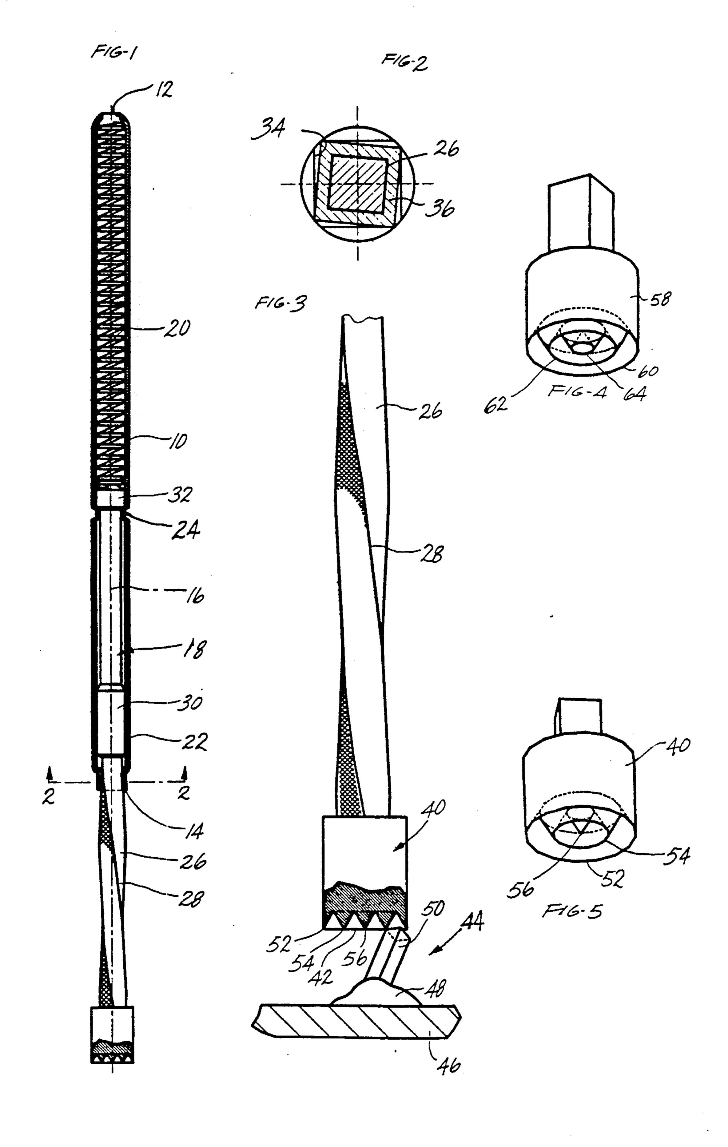
about its axis during probing. By twisting about its axis, the bottom contact tip portion of the probe can bite into the contact point on the unit under test to provide better
