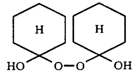
commercial name, Perhexa H 50% Product (Nippon Oils and Fats Co., Ltd.)]are charged into a one liter autoclave and heated to 80° C. while agitating for poly-60 merization over 20 hours to obtain hydroxyl group-containing polyisoprene (yield 65%, Mn = 5,500, OH value 21 mg/g).
