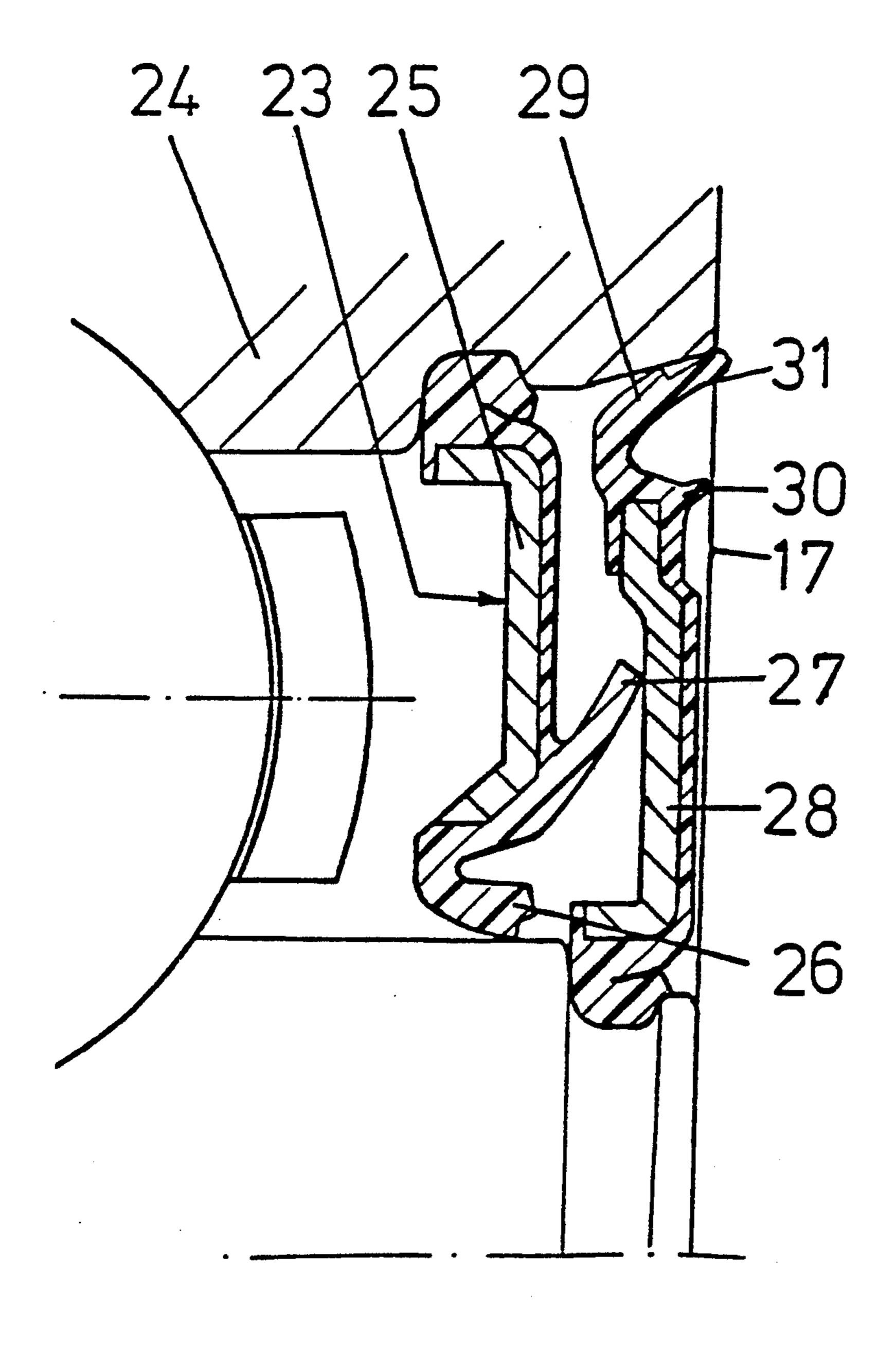
SEAL WITH TWO SEALING RINGS
