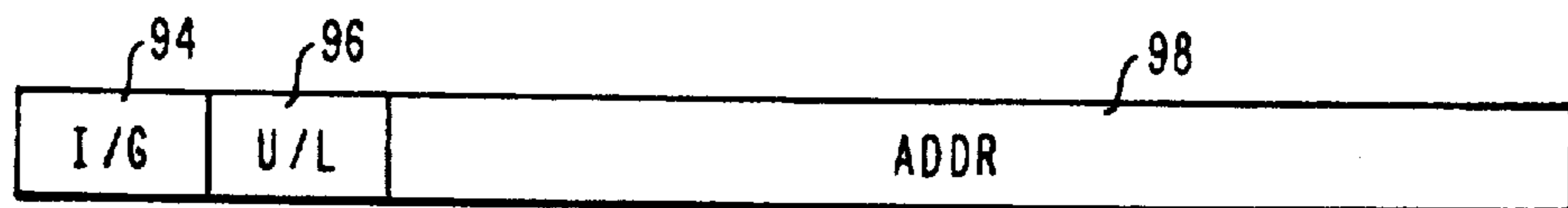
FIG. 6a IEEE 802.3 STANDARD INDIVIDUAL MESSAGE FORMAT
