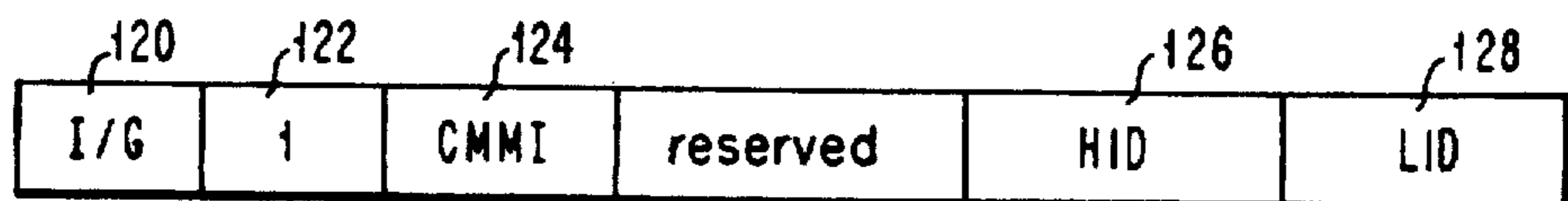
FIG. 7a INDIVIDUAL LOCAL ADDRESS FORMAT
