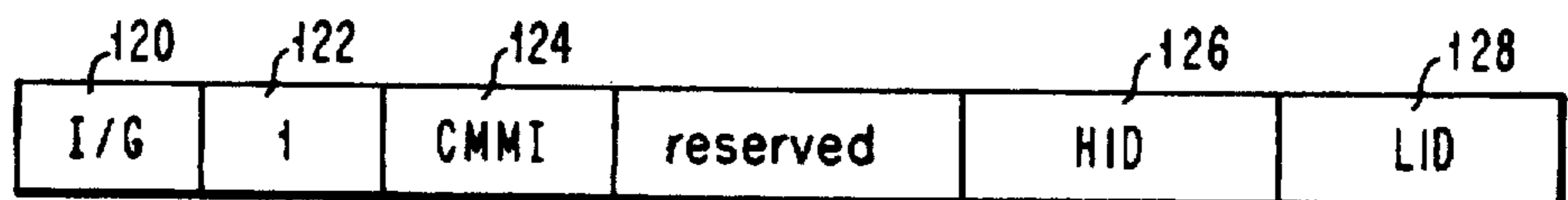
FIG. 7a INDIVIDUAL LOCAL ADDRESS FORMAT
