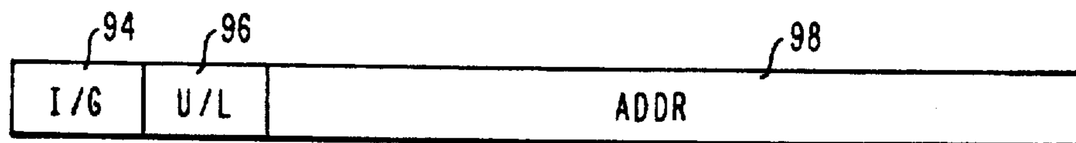
FIG. 6a IEEE 802.3 STANDARD INDIVIDUAL MESSAGE FORMAT
