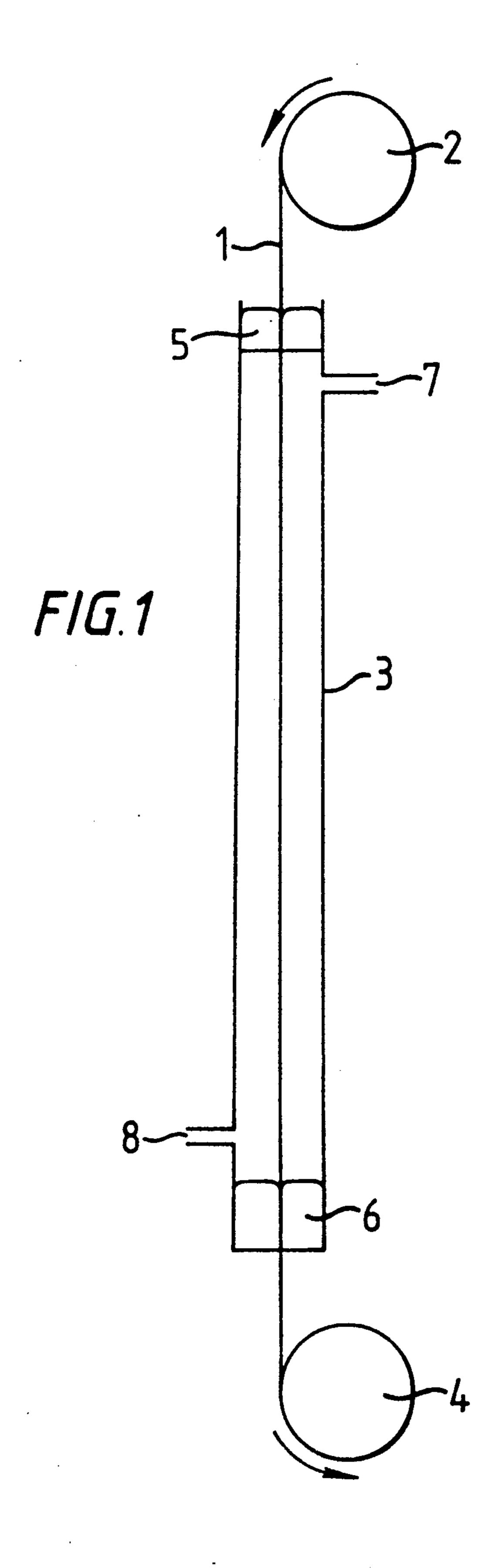
PROCESS FOR DEPOSITING A SILICON CARBIDE COATING ON A FILAMENT
