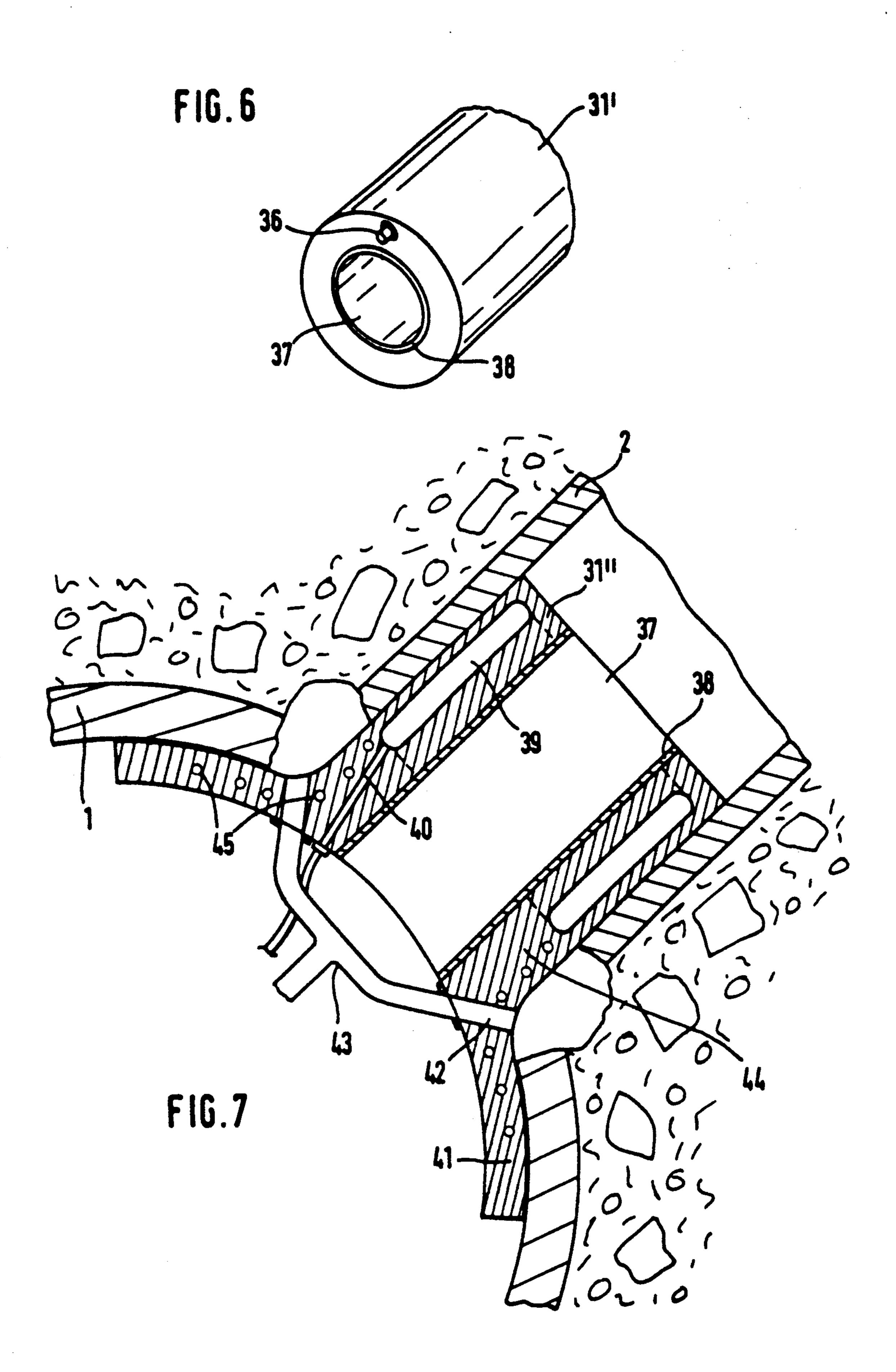
METHOD FOR REPAIRING AN INACCESSIBLE SEWAGE PIPE LEADING AWAY FROM A HOUSE USING A REMOTE-CONTROLLED APPARATUS OPERATING IN THE MAIN SEWAGE PIPE
