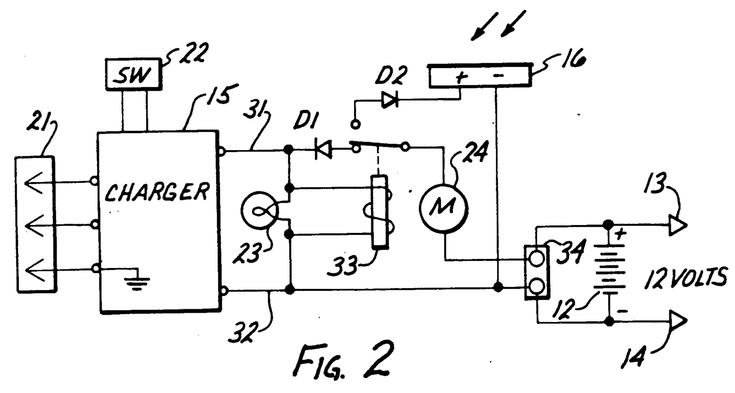
the solar panel from the battery when the charger is powered.
