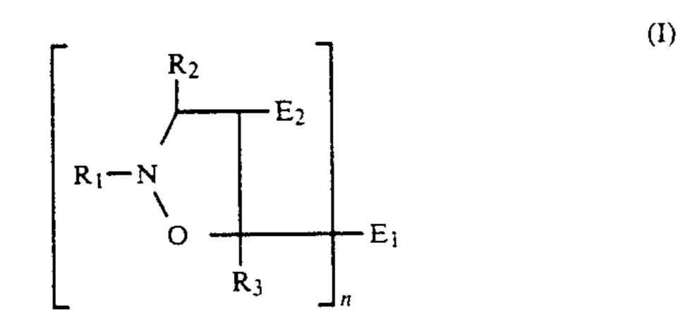
where R<sub>1</sub> and R<sub>2</sub> are independently alkyl, cycloalkyl, alkenyl, aryl or phenylalkyl, R2 is additionally hydrogen, R<sub>3</sub> is hydrogen or methyl, n is 1-4, E<sub>1</sub> is an electron withdrawing group, and E2 is hydrogen, alkyl, phenyl or has the same meaning as E1, are effective in stablizing organic materials against oxidative, thermal and actinic degradation.
