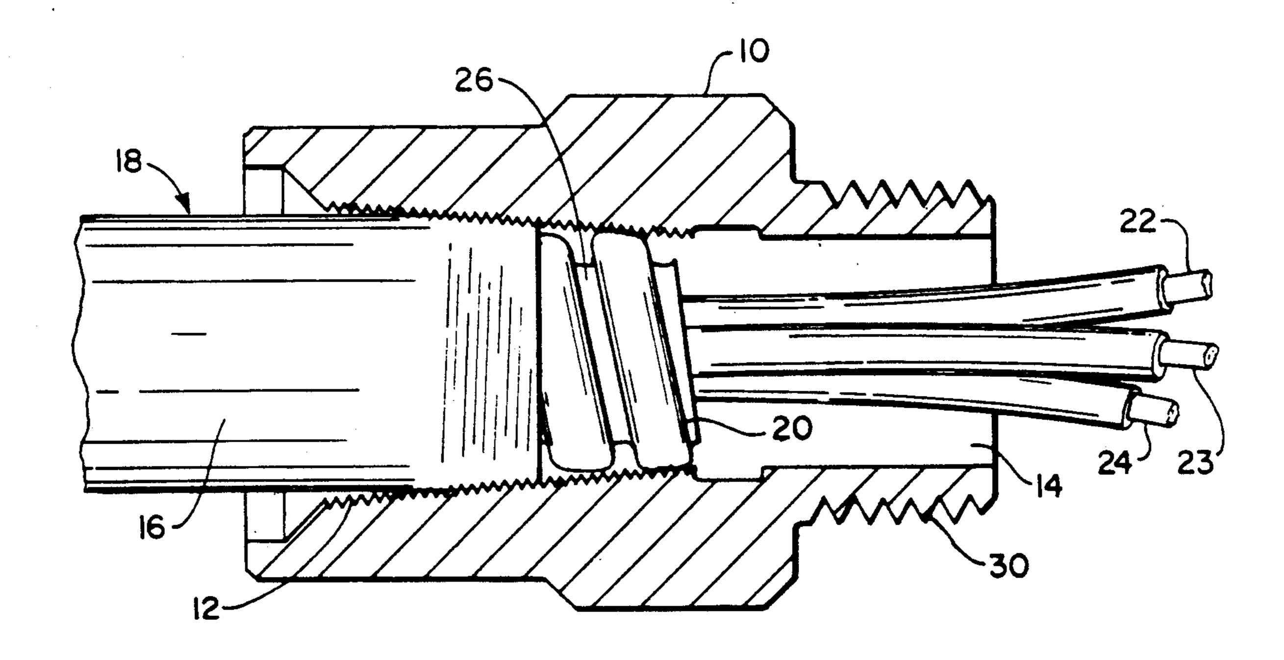
Another object of the invention is to provide a ground connection between the metal clad of the con-CONNECTOR FOR JOINING JUNCTION AND duit and the box. PANEL BOXES TO METAL CLAD JACKETED
