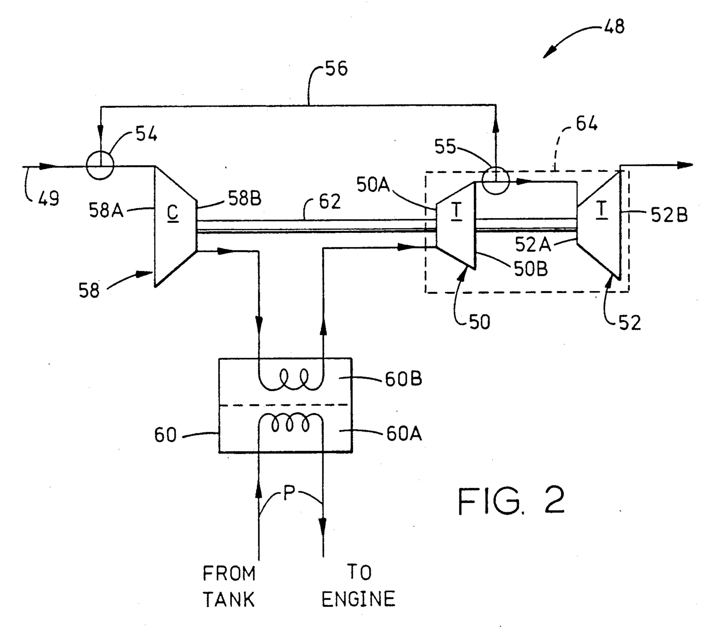
AUXILIARY REFRIGERATED AIR SYSTEM EMPLOYING MIXTURE OF AIR BLED FROM TURBINE ENGINE COMPRESSOR AND AIR RECIRCULATED WITHIN AUXILIARY SYSTEM
