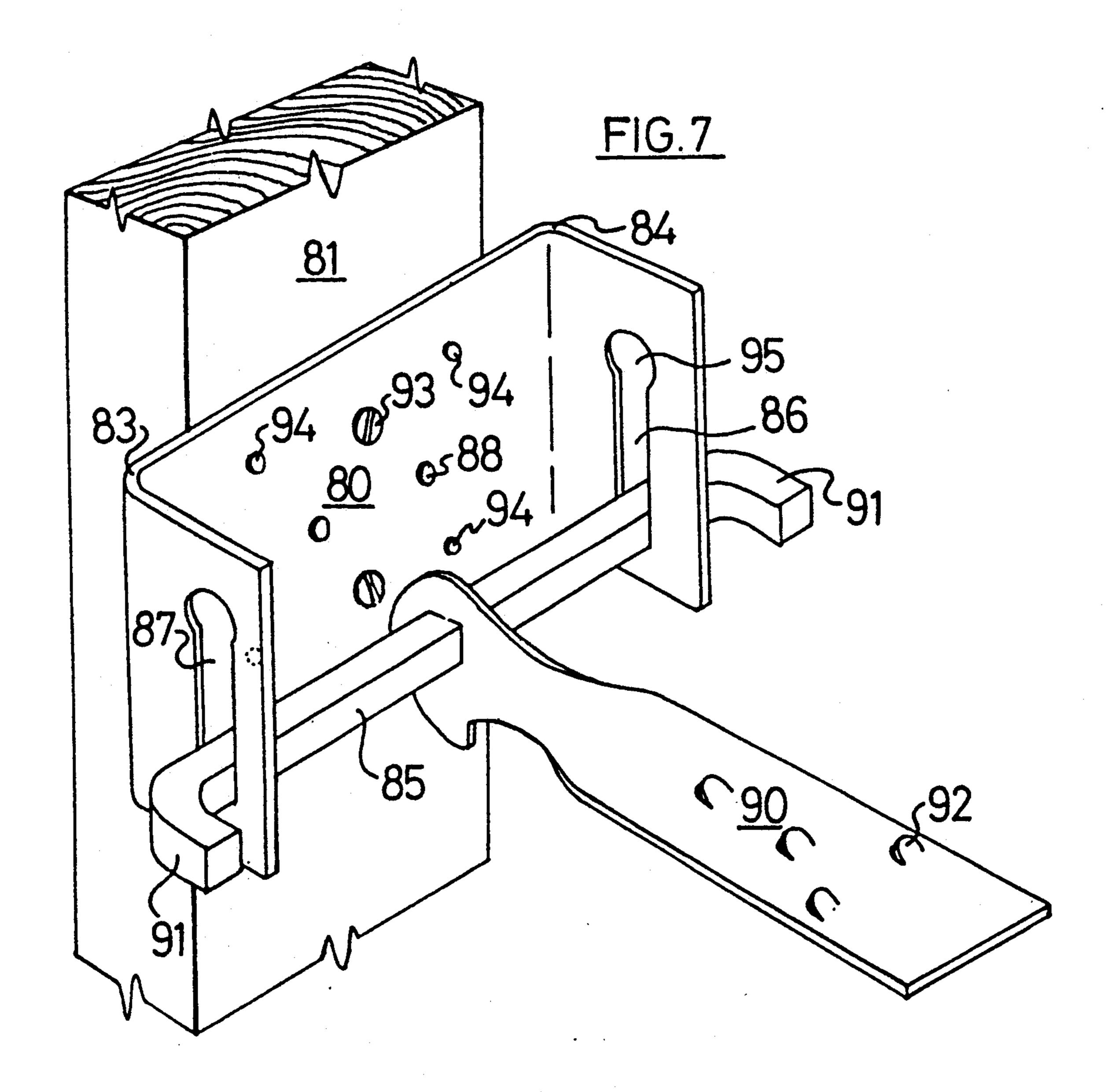
tomer between two channels, so that the two channels are resiliently connected together and also insulated one from the other.
