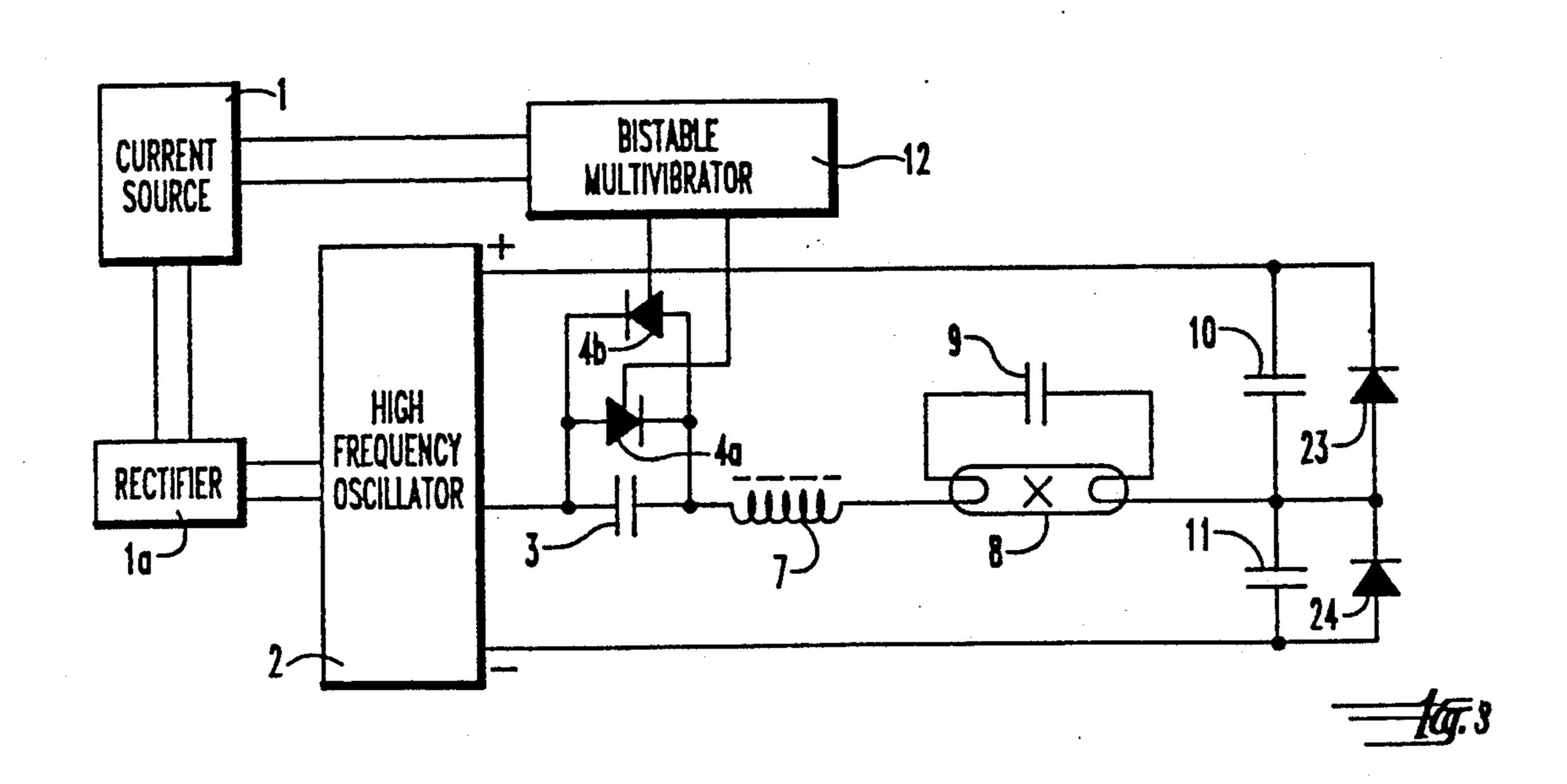
METHOD OF AND APPARATUS FOR SUPPLYING HIGH FREQUENCY ALTERNATING CURRENT TO A FLUORESCENCE LAMP
