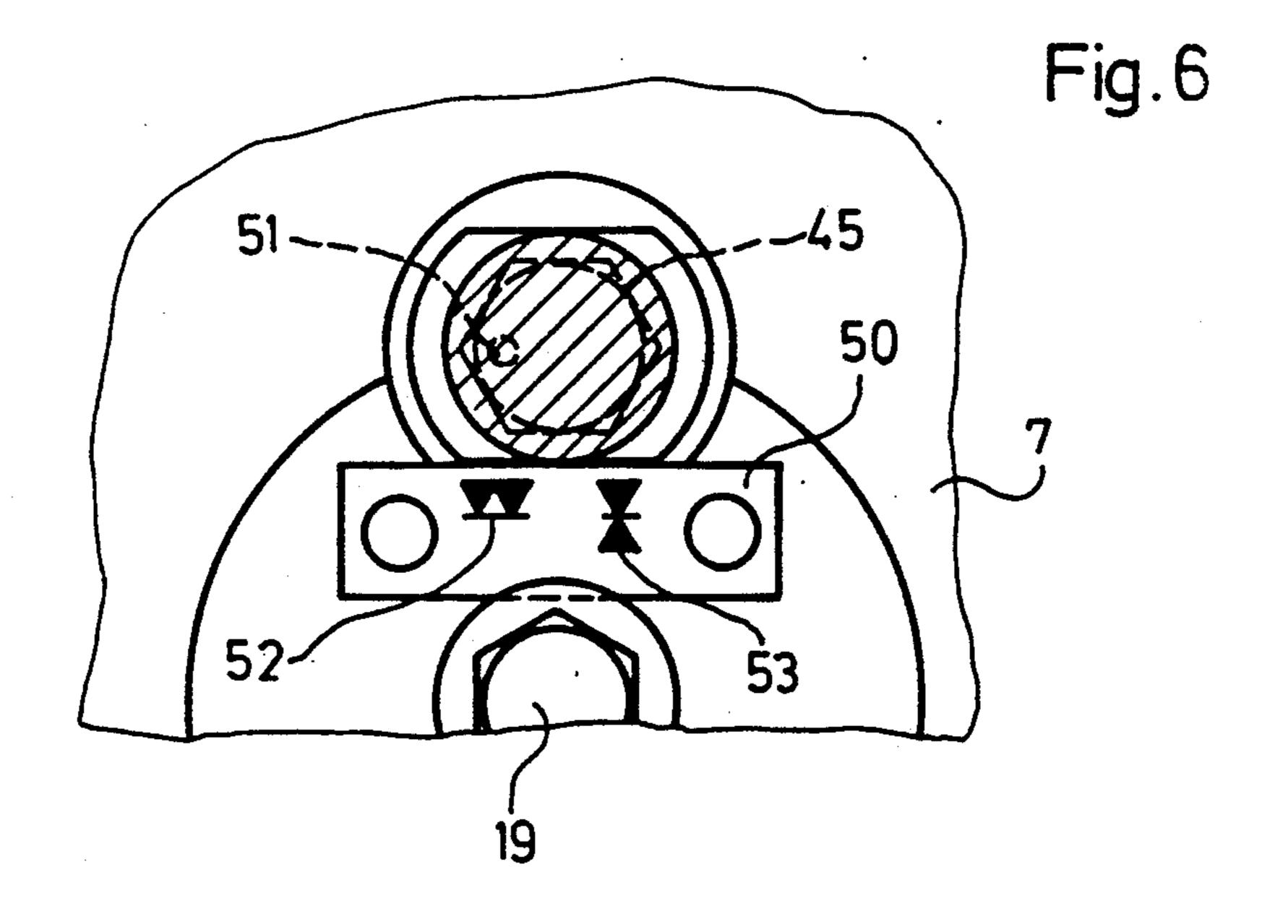
the hereinafore-mentioned safety device of the device for clamping the fixed gear and the adjusting gear together.
