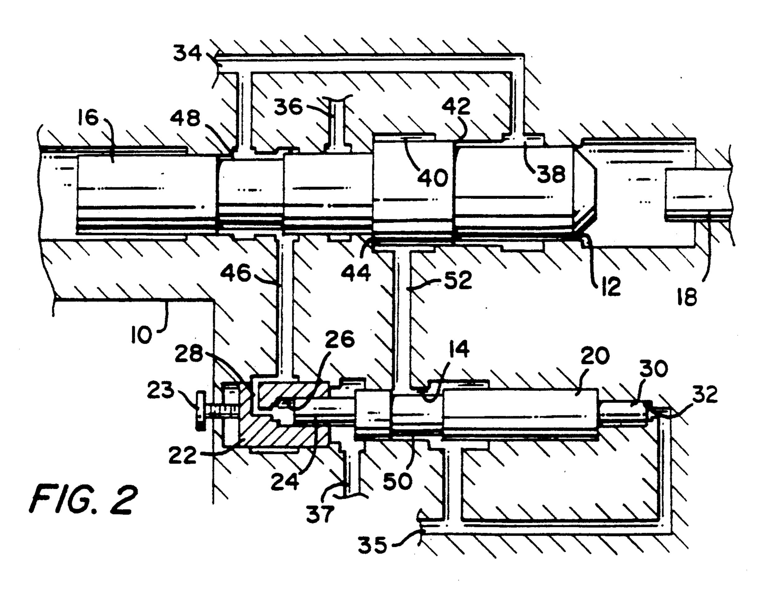
actuator of the instant invention, with the piston 16 being displayed positioned to the right of its stroke; VARIABLE FREQUENCY CONTROL FOR
