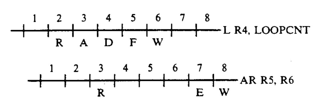
However, a timing chart for this instruction sequence, using the instruction stack of FIG. 4, in accordance with the present invention, is set forth below:
