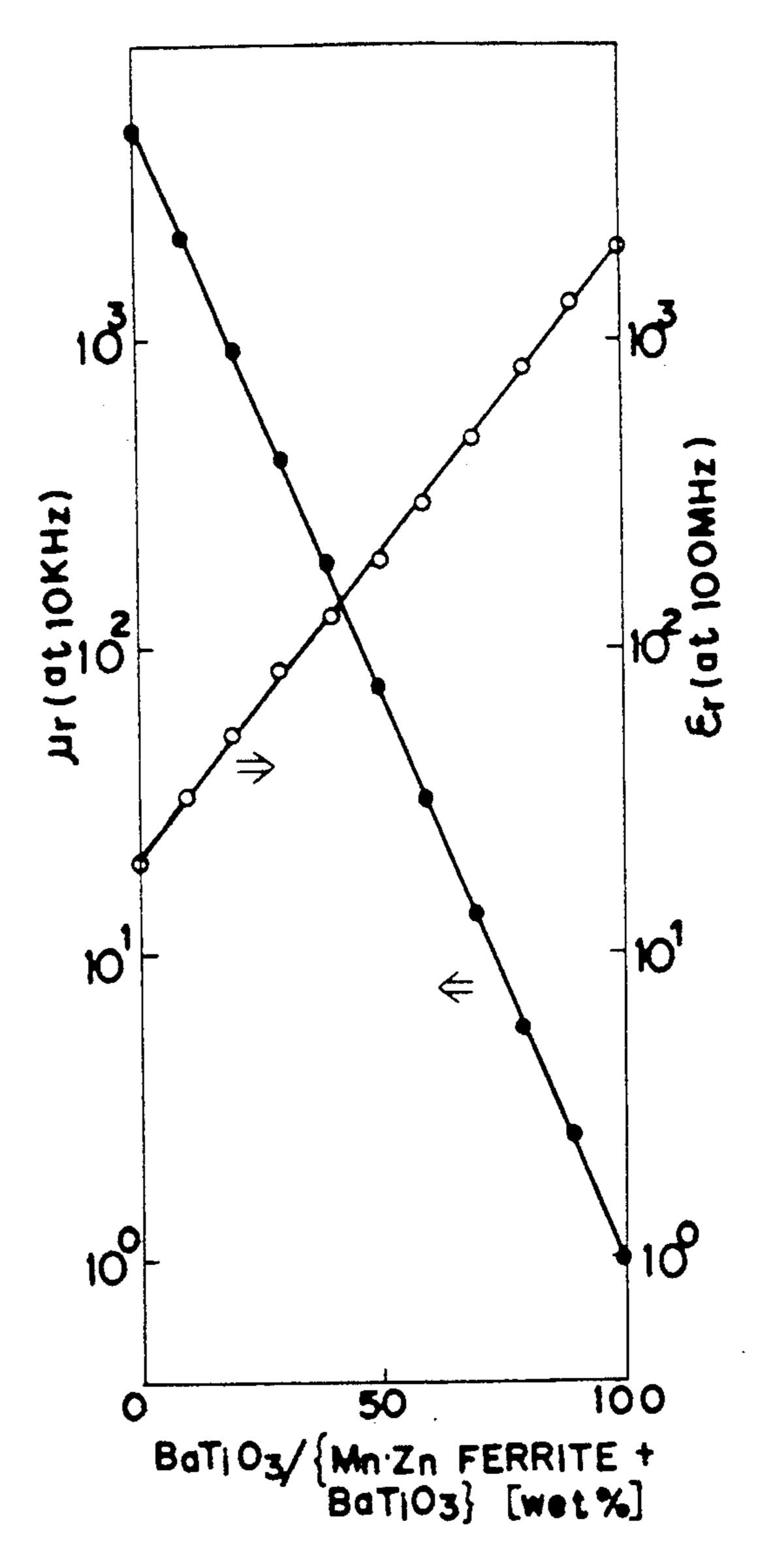
BaTiO<sub>3</sub> - Mn·Zn FERRITE (MnO:ZnO:Fe<sub>2</sub>O<sub>3</sub>= 0.225:022:0525)
