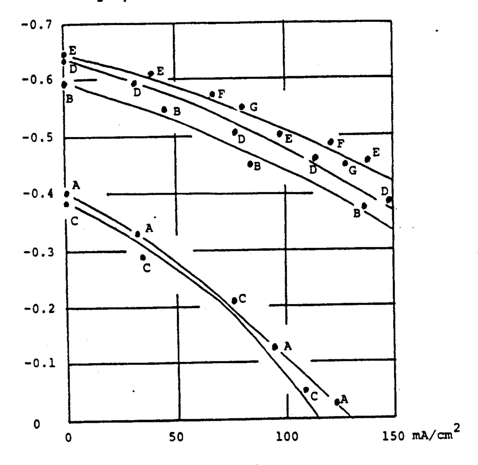
Figure 1. Voltage-current curves vs reference electrode at 60 °C in 4-M H<sub>2</sub>SO<sub>4</sub> and 1-M MeOH. The base formulation is 0.7 mg Pt + 0.7 mg Ru per cm2. Experimental data refer to following conditions: A added lead 0 mg Pb/cm<sup>2</sup>, BQ.7 mg Pb/cm<sup>2</sup> after 1 week, C as B but 3 weeks, D 1.0 mg Pb/cm<sup>2</sup> after 3 weeks, E as D but 1.5 mg Pb/cm<sup>2</sup>, F as D but 5.0 mg Pb/cm<sup>2</sup> and G as D but 10.0 mg Pb/cm<sup>2</sup>.
