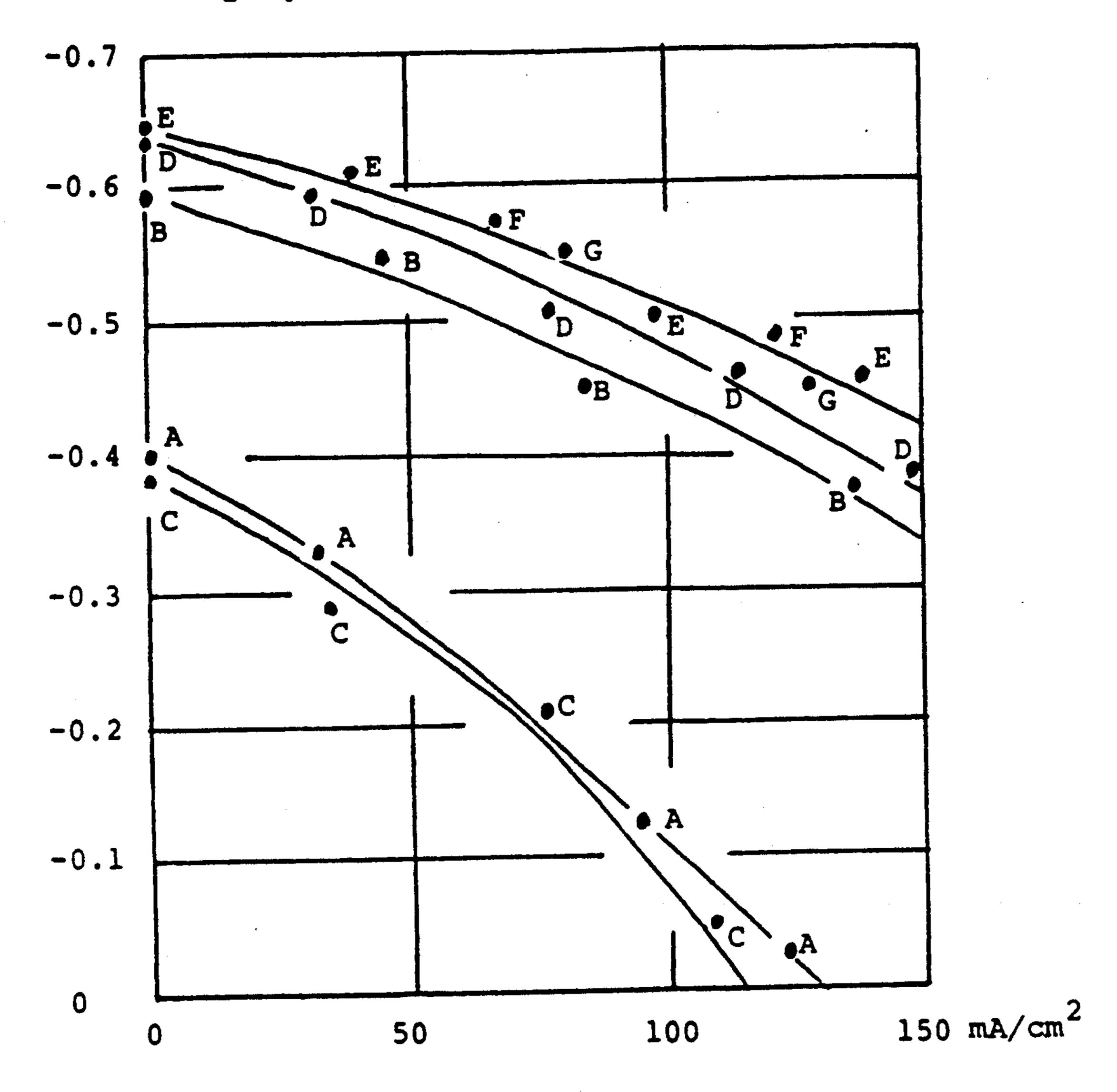
Figure 1. Voltage-current curves vs reference electrode at 60 °C in 4-M H<sub>2</sub>SO<sub>4</sub> and 1-M MeOH. The base formulation is 0.7 mg Pt + 0.7 mg Ru per cm<sup>2</sup>. Experimental data refer to following conditions: A added lead 0 mg Pb/cm<sup>2</sup>, B 0.7 mg Pb/cm<sup>2</sup> after 1 week, C as B but 3 weeks, D 1.0 mg Pb/cm<sup>2</sup> after 3 weeks, E as D but 1.5 mg Pb/cm<sup>2</sup>, F as D but 5.0 mg Pb/cm<sup>2</sup> and G as D but 10.0 mg Pb/cm<sup>2</sup>.
