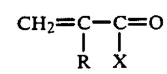
wherein R is hydrogen or methyl and X is OR' or NR<sub>2</sub>" in which R' is hydrogen, C<sub>1</sub>-C<sub>18</sub> alkyl or cycloalkyl, 2-hydroxethyl, hydroxypropyl, hydroxybutyl or 2-cyanoethyl, and R" is hydrogen, methyl or CH<sub>2</sub>OR" in which R" is hydrogen, methyl, ethyl, propyl or butyl.
