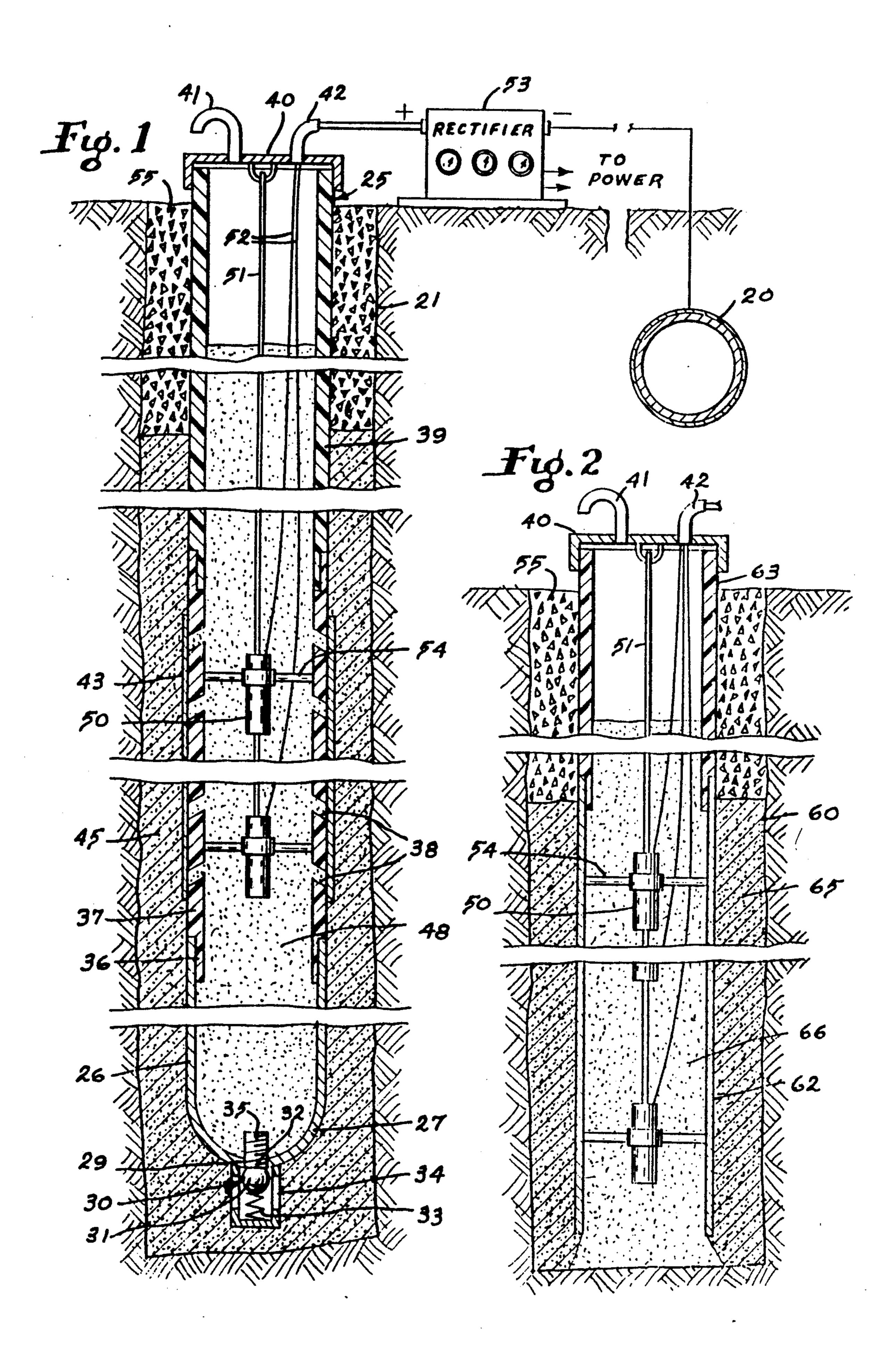
GROUND ELECTRODE BACKFILL COMPOSITION, ANODE BED
