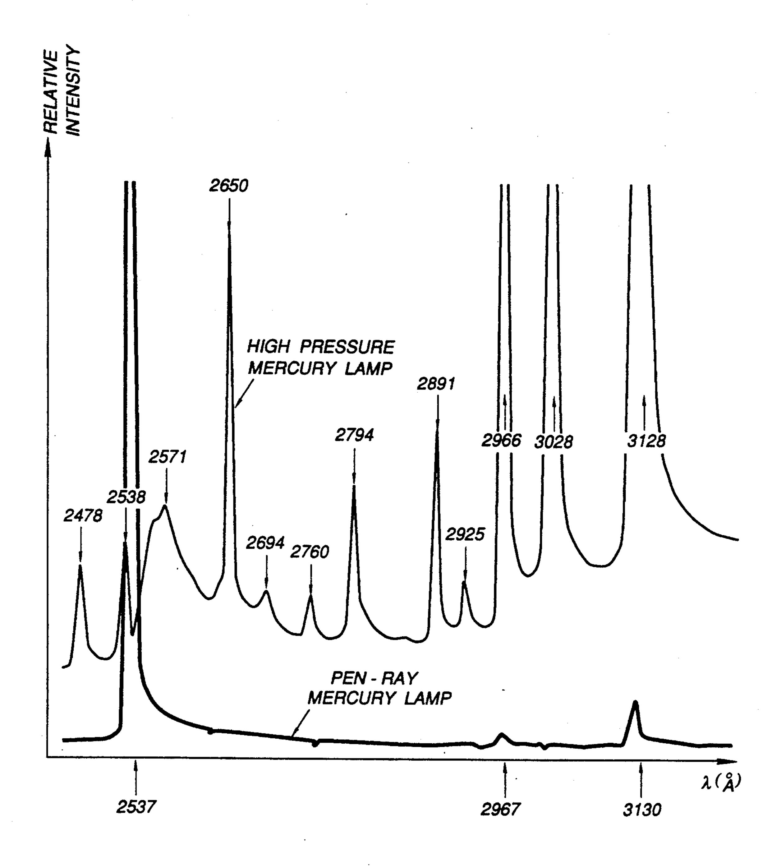
Spectrum of the high pressure mercury lamp and Pen - ray lamp.
