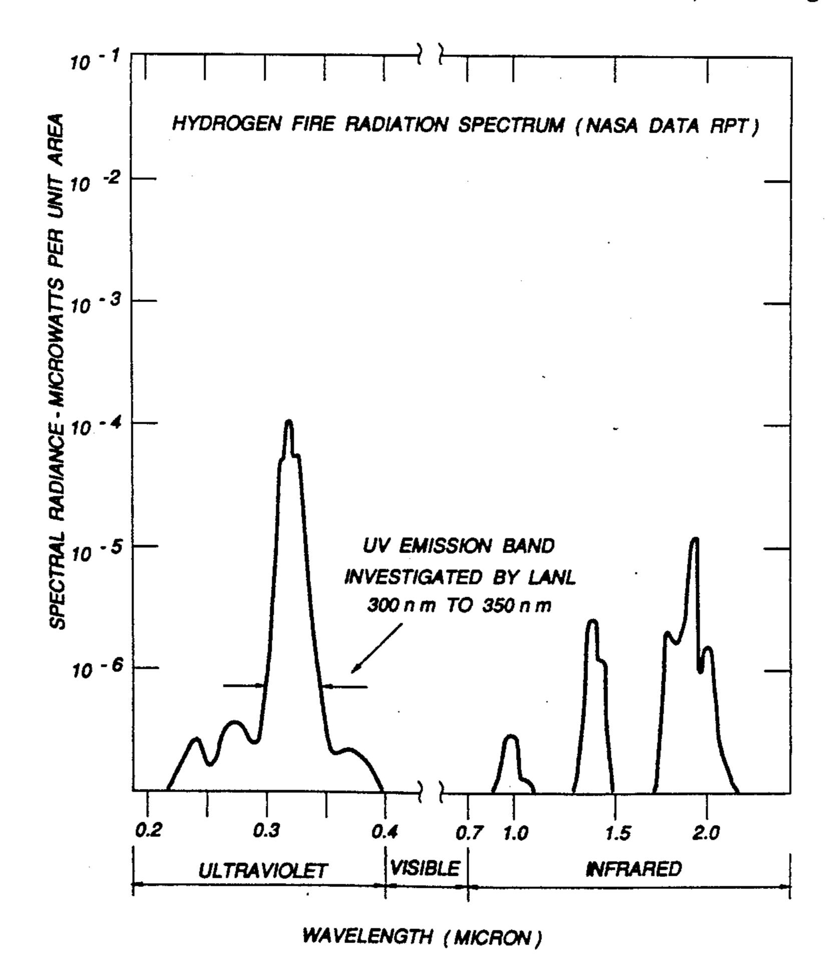
Hydrogen fire radiation spectrum, replotted from data supplied by NASA.
