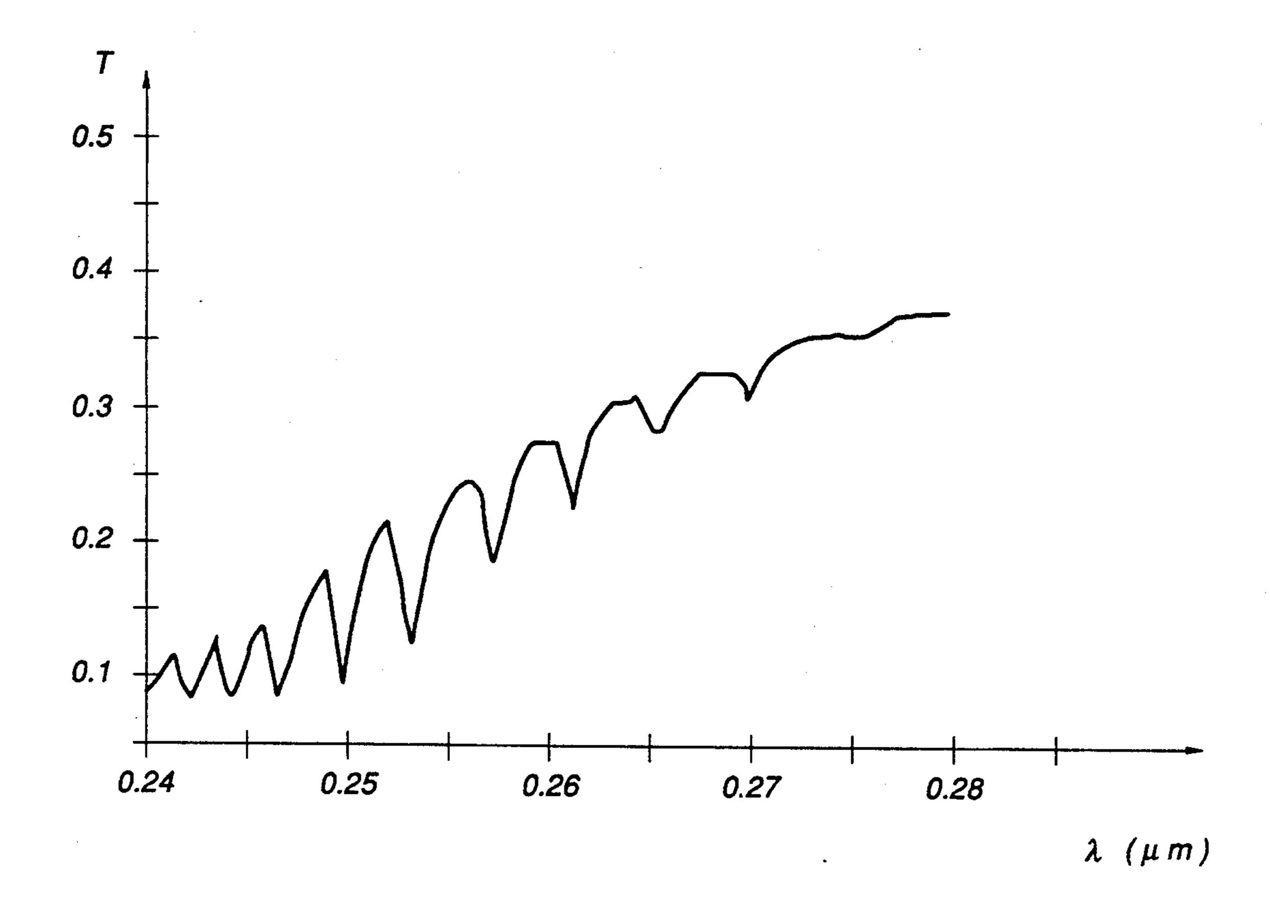
Atmospheric transmittance in middle UV over 1 Km horizontal path under typical atmospheric conditions.
