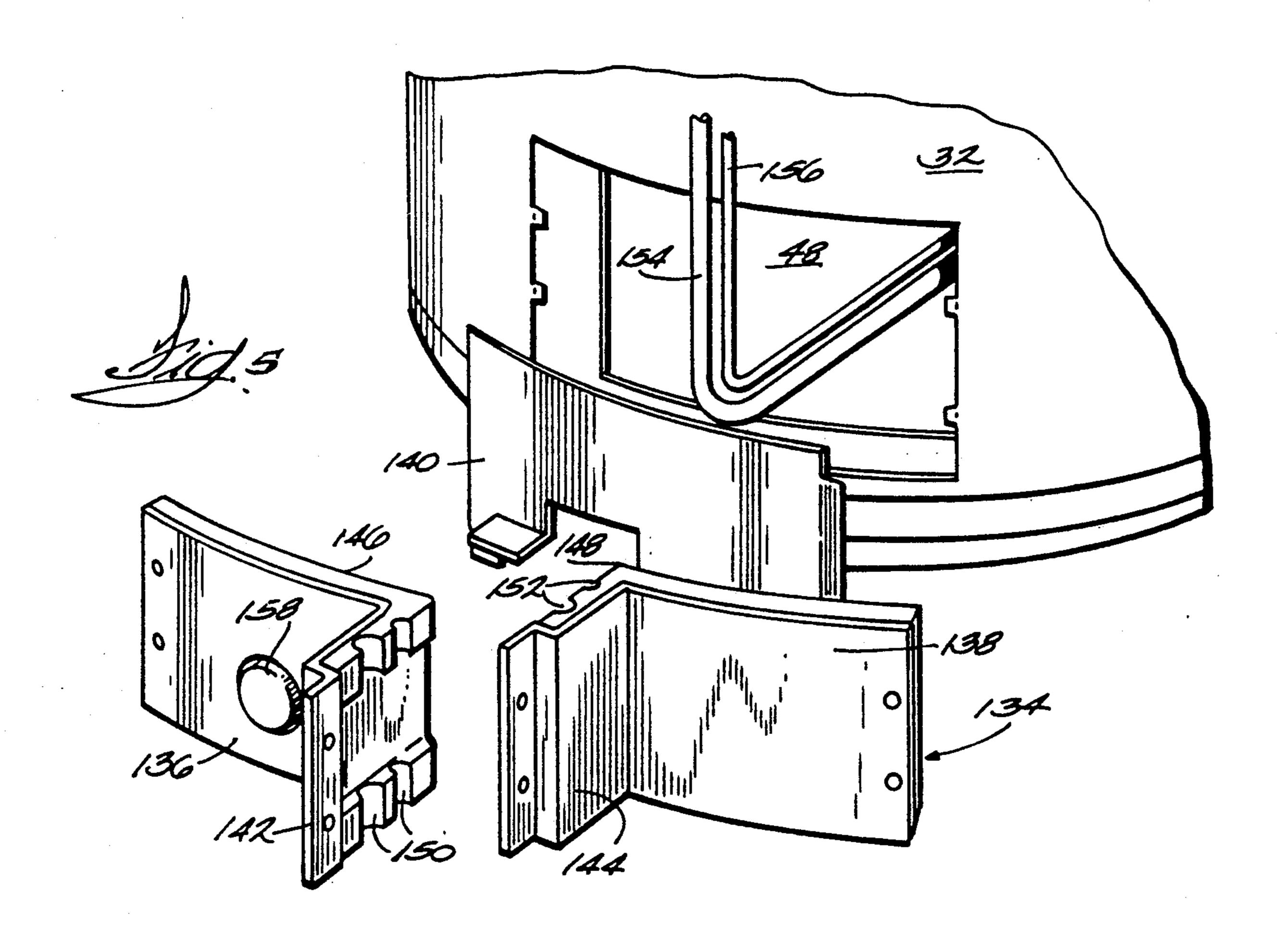
FIG. 6 is a perspective view of the access door assembly in its assembled position.
