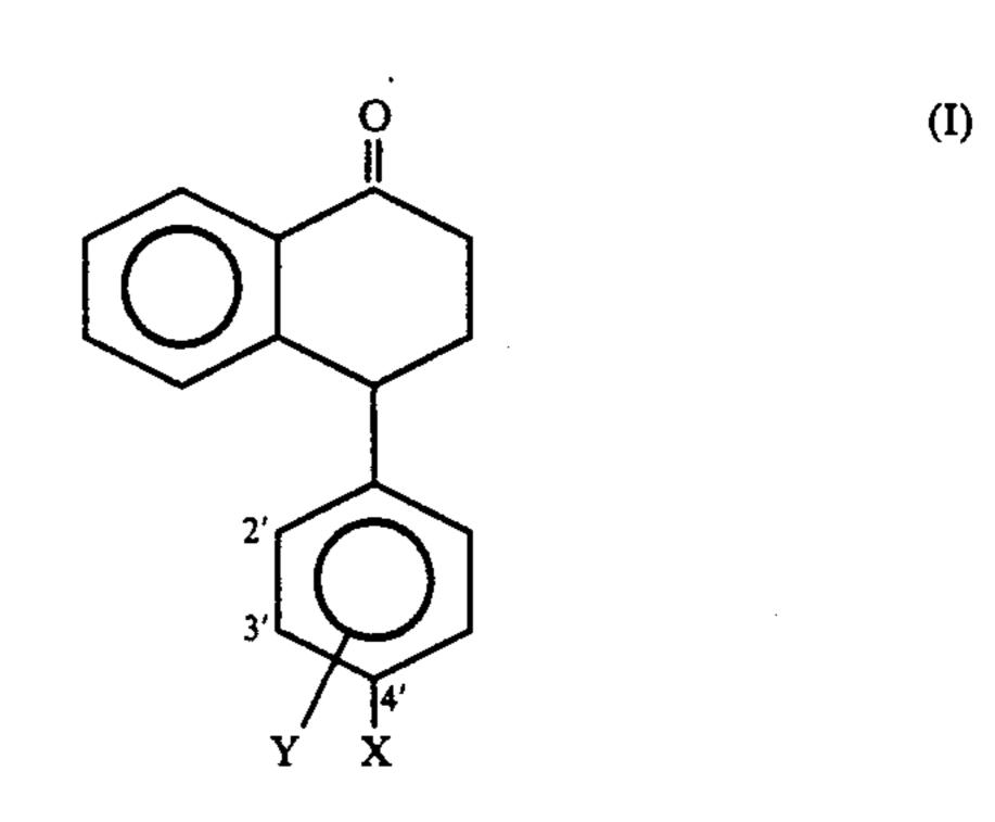
in which X represents halogen,  $C_1$ – $C_4$  alkyl or  $C_1$ – $C_4$  alkoxy and Y, situated in position 2' or 3', represents halogen or  $C_1$ – $C_4$  alkyl, this method being characterized in that it comprises the reaction, in the presence of an acid agent, of  $\alpha$ -naphthol of formula (II) with a phenyl compound of formula (III):
