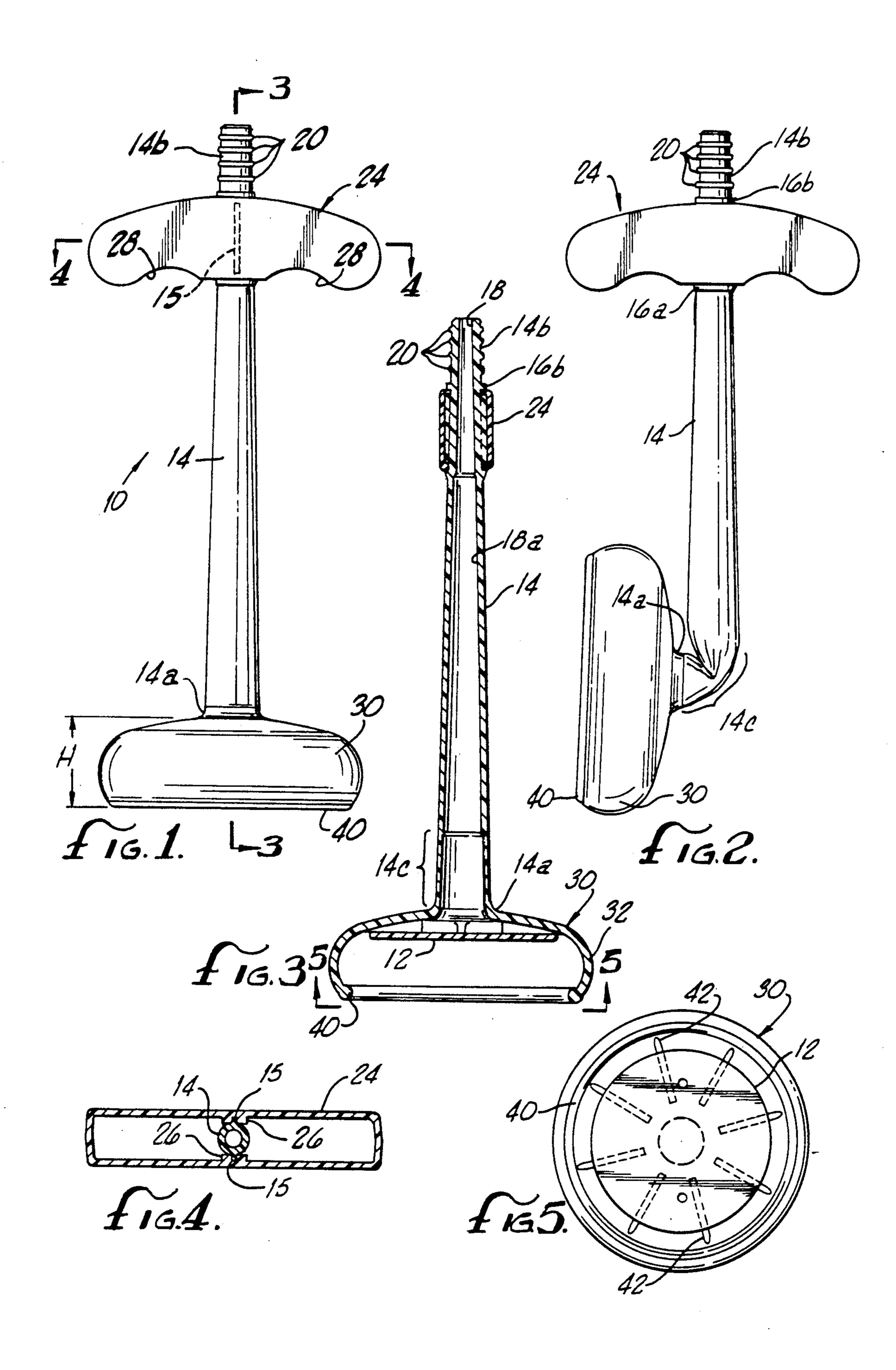
FIG. 3 is a cross-sectional view of the handle of FIG. 1 taken along line 3—3;
