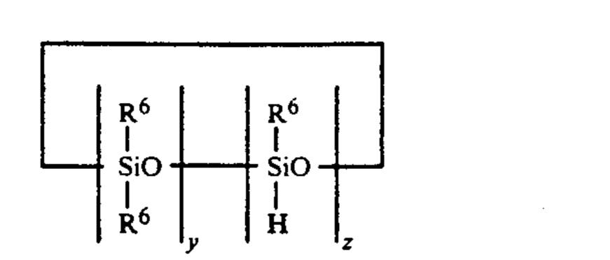
wherein R<sup>6</sup> may be independently hydrogen, an alkyl radical of from 1 to 8 carbon atoms, an aryl radical from 6 to 14 carbon atoms, or a haloalkyl radical of 3 to 8 carbon atoms; y is an integer having a value of 0 to 5 inclusive, z is an integer having a value of from 1 to 8 inclusive, and the sum of y and z has a value of 3 to 8 inclusive.
