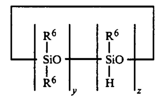
wherein R<sup>6</sup> may be independently hydrogen, an alkyl radical of from 1 to 8 carbon atoms, an aryl radical from 6 to 14 carbon atoms, or a haloalkyl radical of 3 to 8 carbon atoms; y is an integer having a value of 0 to 5 inclusive, z is an integer having a value of from 1 to 8 inclusive, and the sum of y and z has a value of 3 to 8 inclusive; and
