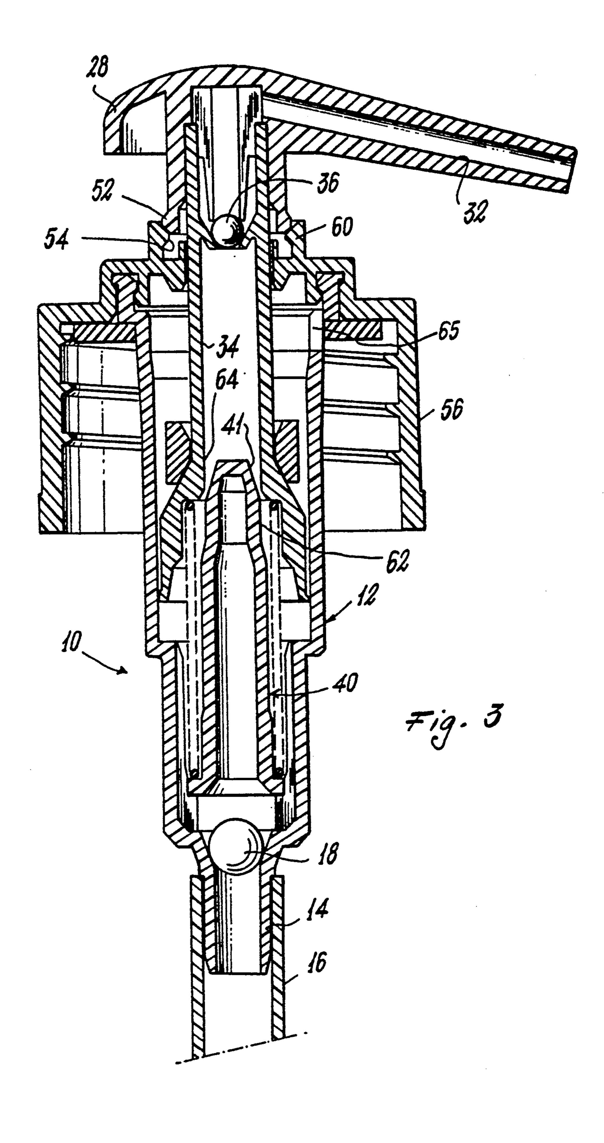
HAND PUMP FOR DISPENSING BOTTLES WITH SHUTOFF ARRANGEMENT FOR PREVENTING SPILLAGE THEREFROM
