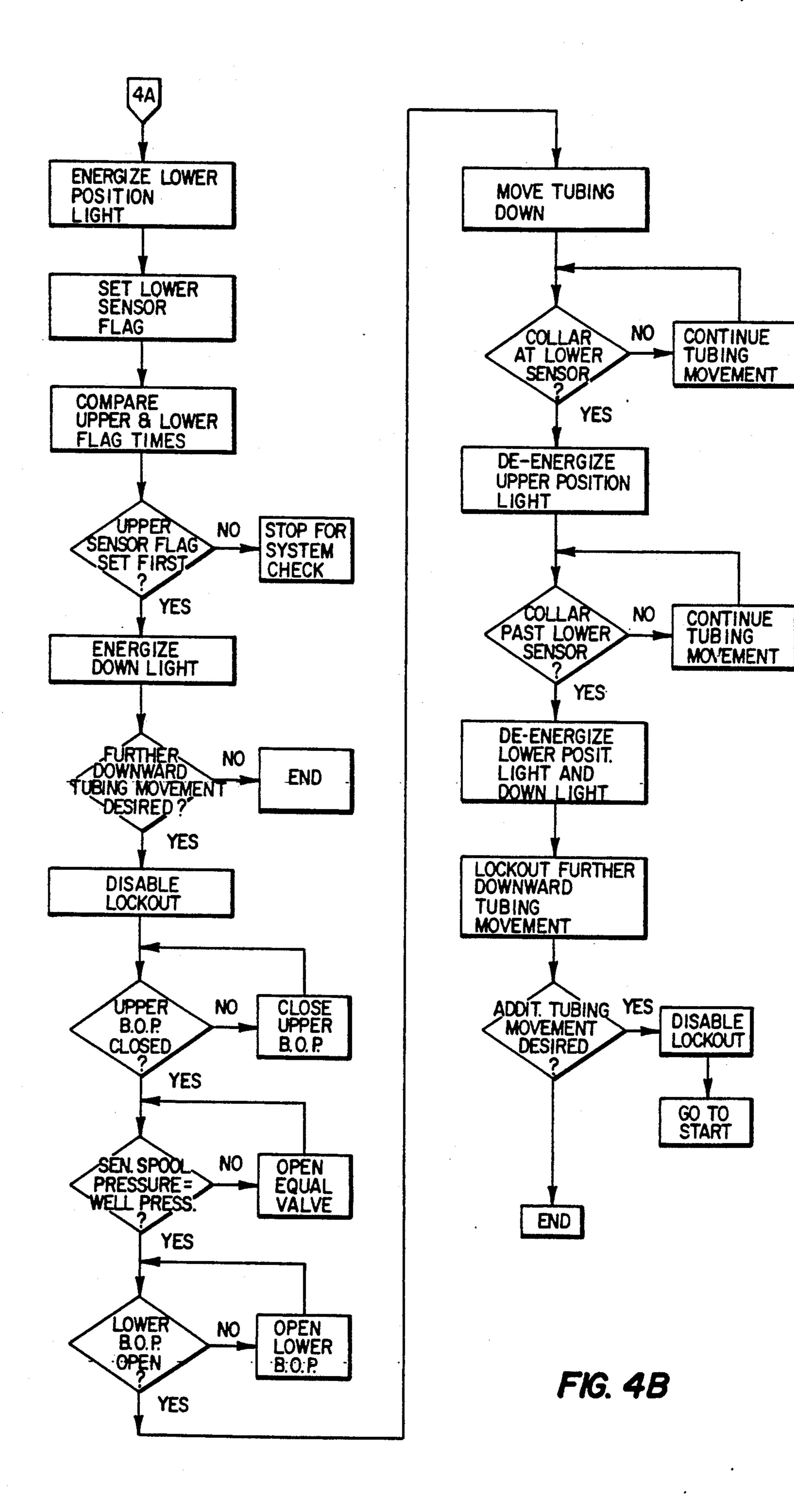
TUBING COLLAR POSITION SENSING APPARATUS, AND ASSOCIATED METHODS, FOR **USE WITH A SNUBBING UNIT**
