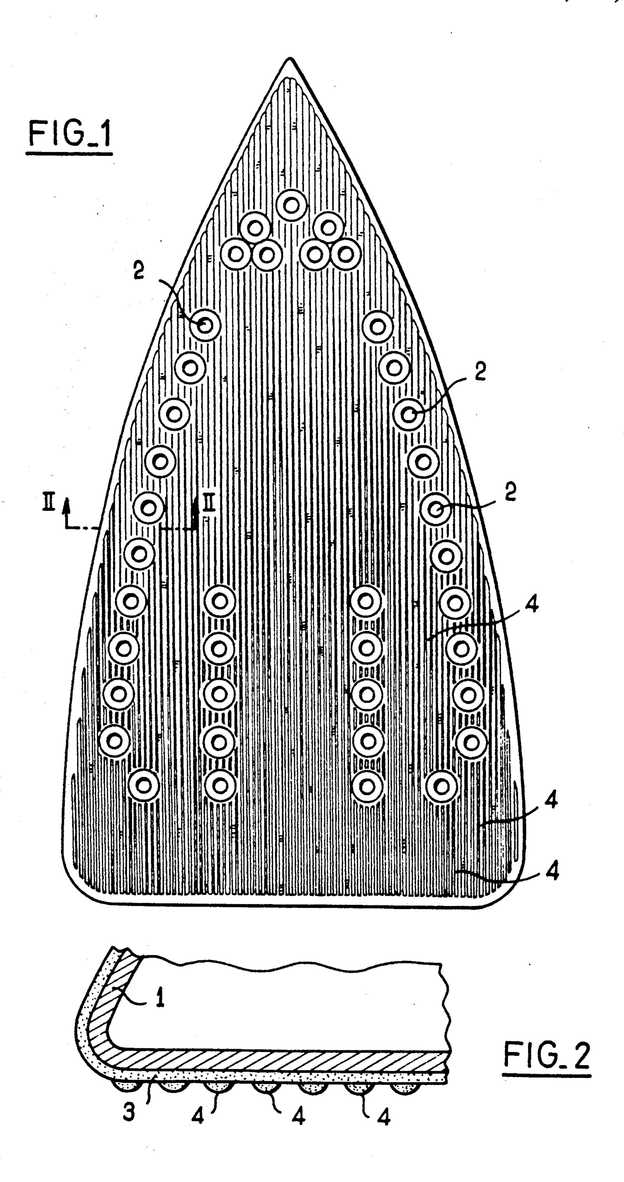
SMOOTHING IRON HAVING SCREEN PRINTED ENAMEL STRIPS WIDER AT THE FRONT AND NARROWER AT THE REAR OF THE PRESSING SOLE SURFACE
