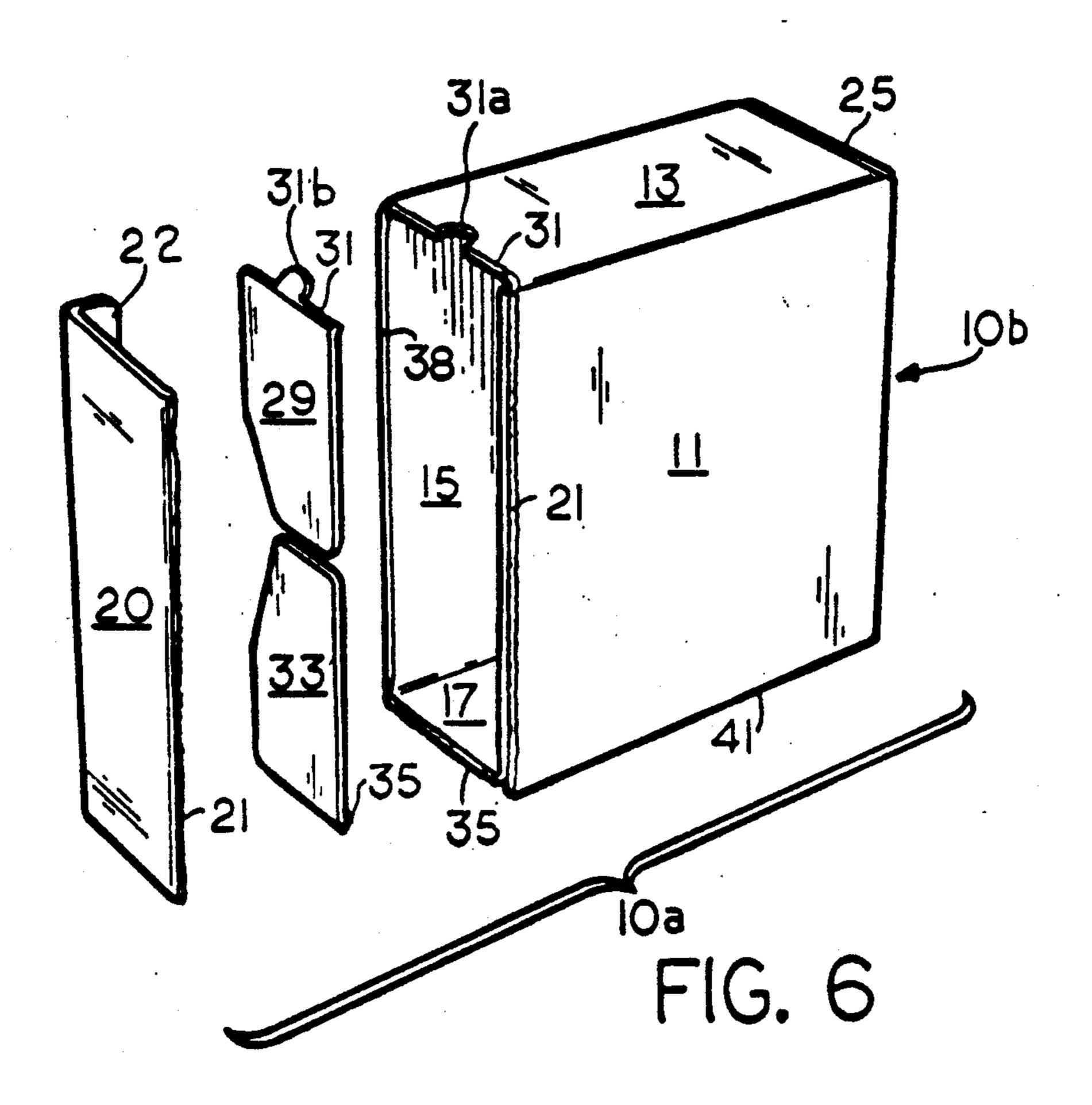
FIG. 6 is a spacial perspective view of the carton of FIG. 5 showing the one end wall torn away along the perforations of the multiple flaps leaving a case for storage of the contents on a book shelf with the one end open and exposed for viewing the contents.
