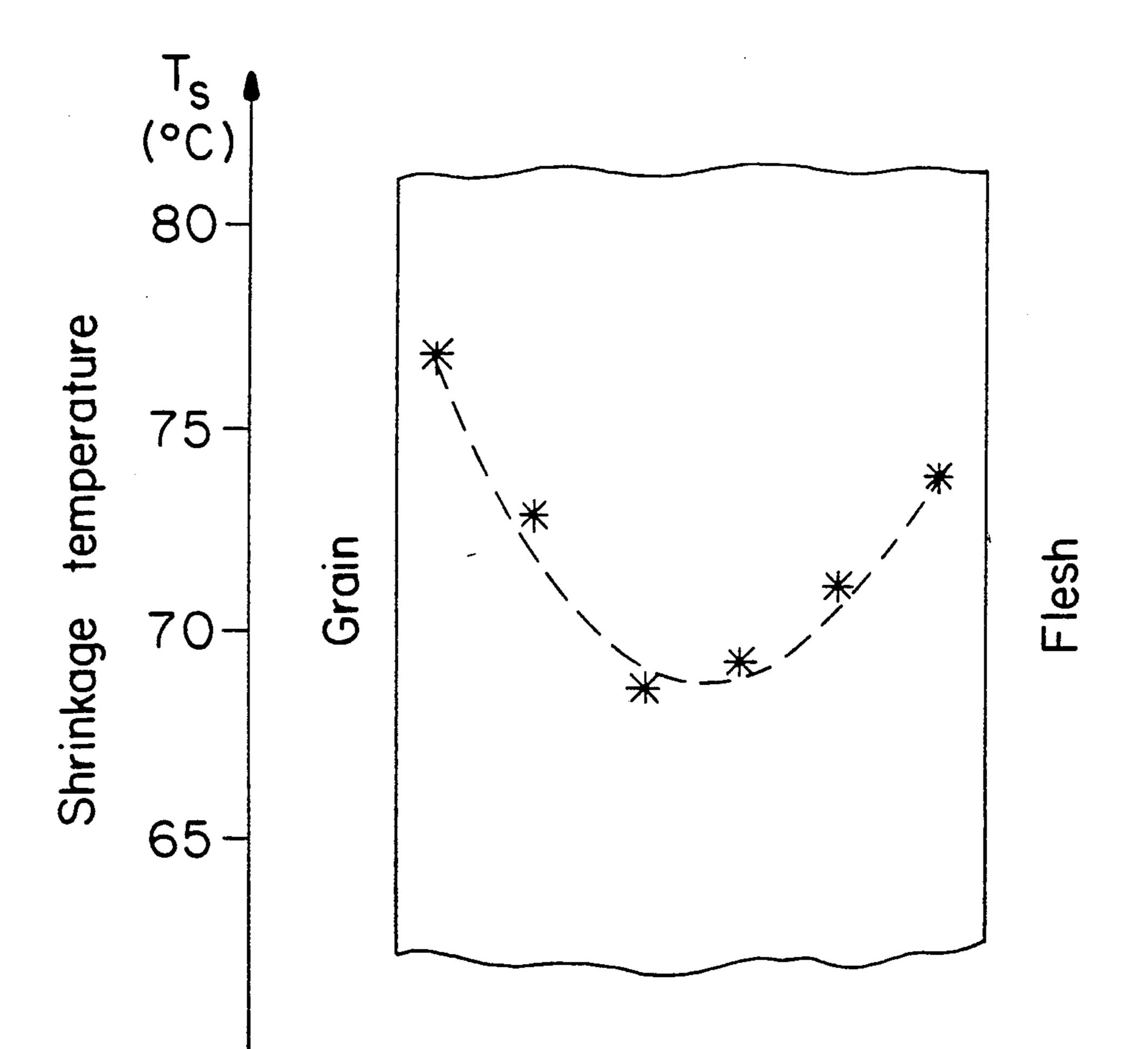
Thermal stability ( $T_s$ ) in the leather cross-section after treatment with 0.5% of glutar-dialdehye, based on 100% strength aldehyde and based on pelt weight.
