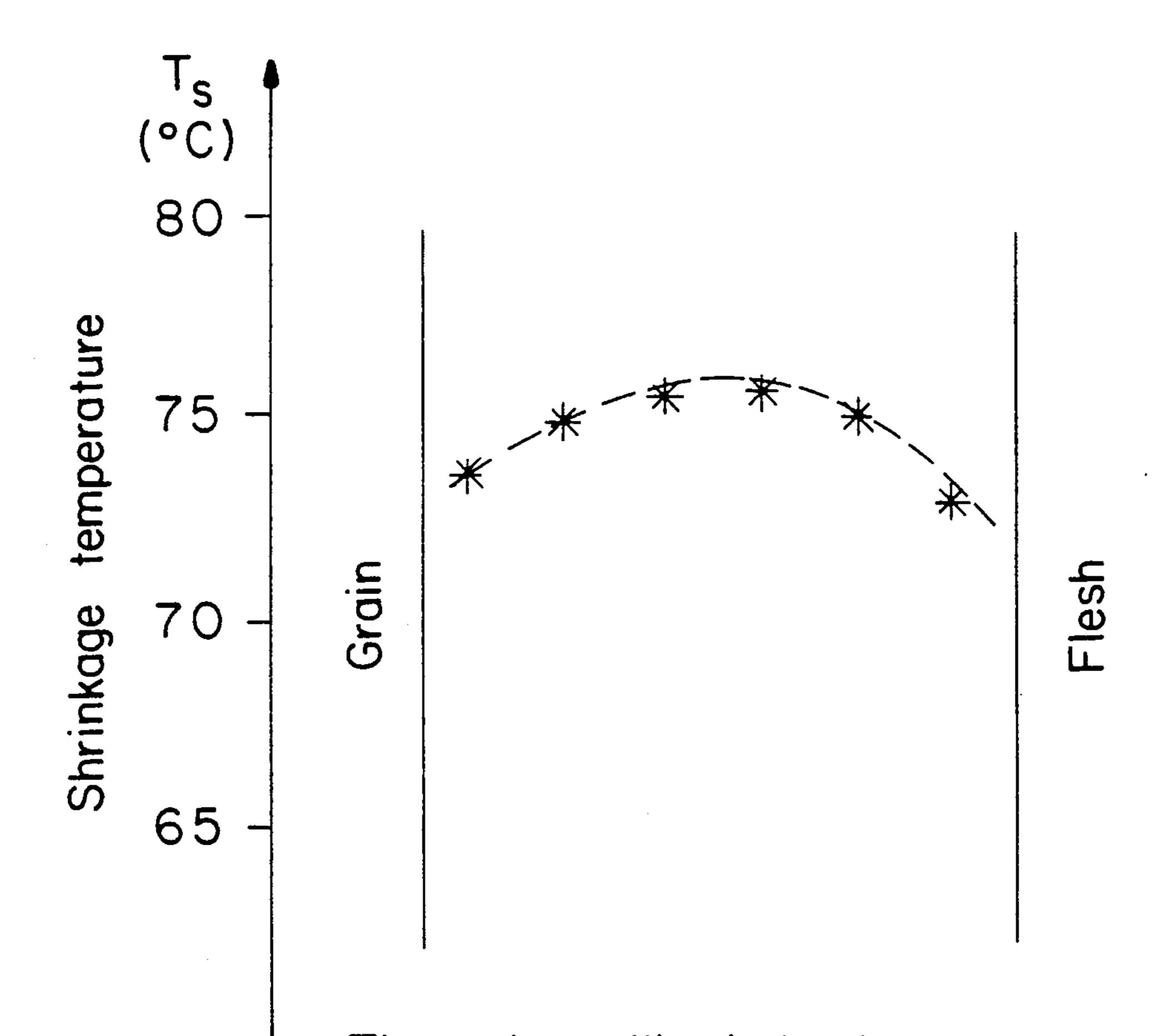
Thermal stability in leather cross-section after treatment with the formulation according to the invention based on technical grade glutardialdehyde (0.5% based on 100% of glutardialdehyde present in the formulation and based on pelt weight).
