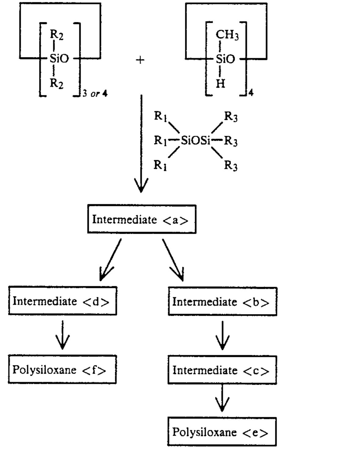
The ultraviolet-hardenable adhesive of the invention 30 preferably contains at least one adjusting constituent for adjusting a bonding force produced by the adhesive. The at least one adjusting constituent is selected from polysiloxanes represented by the following general formula (II):
