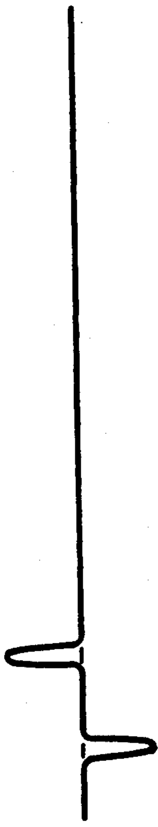
FIG. 6(a) OUTPUT OF REFERENCE-SIGNAL PICK-UP COIL 1
