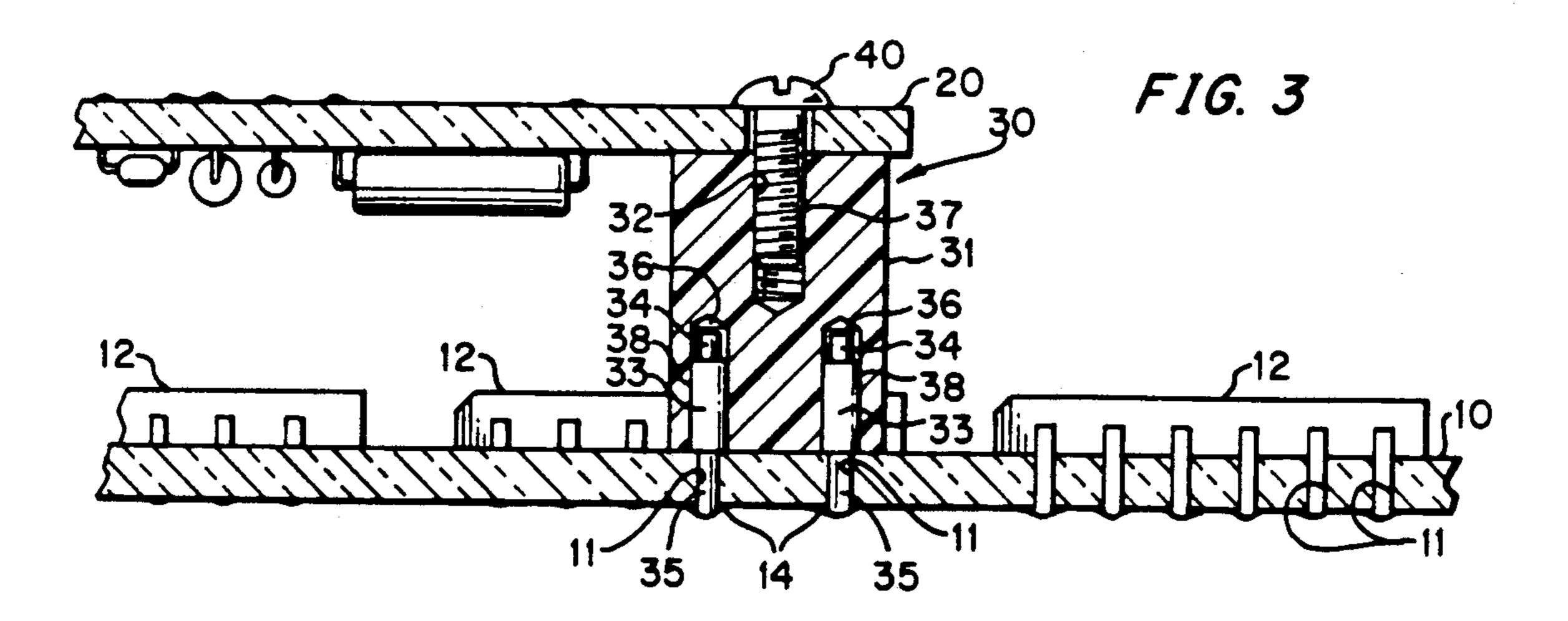
this spacer can be employed with single-sided, double-sided, and multilayer printed circuit boards.
