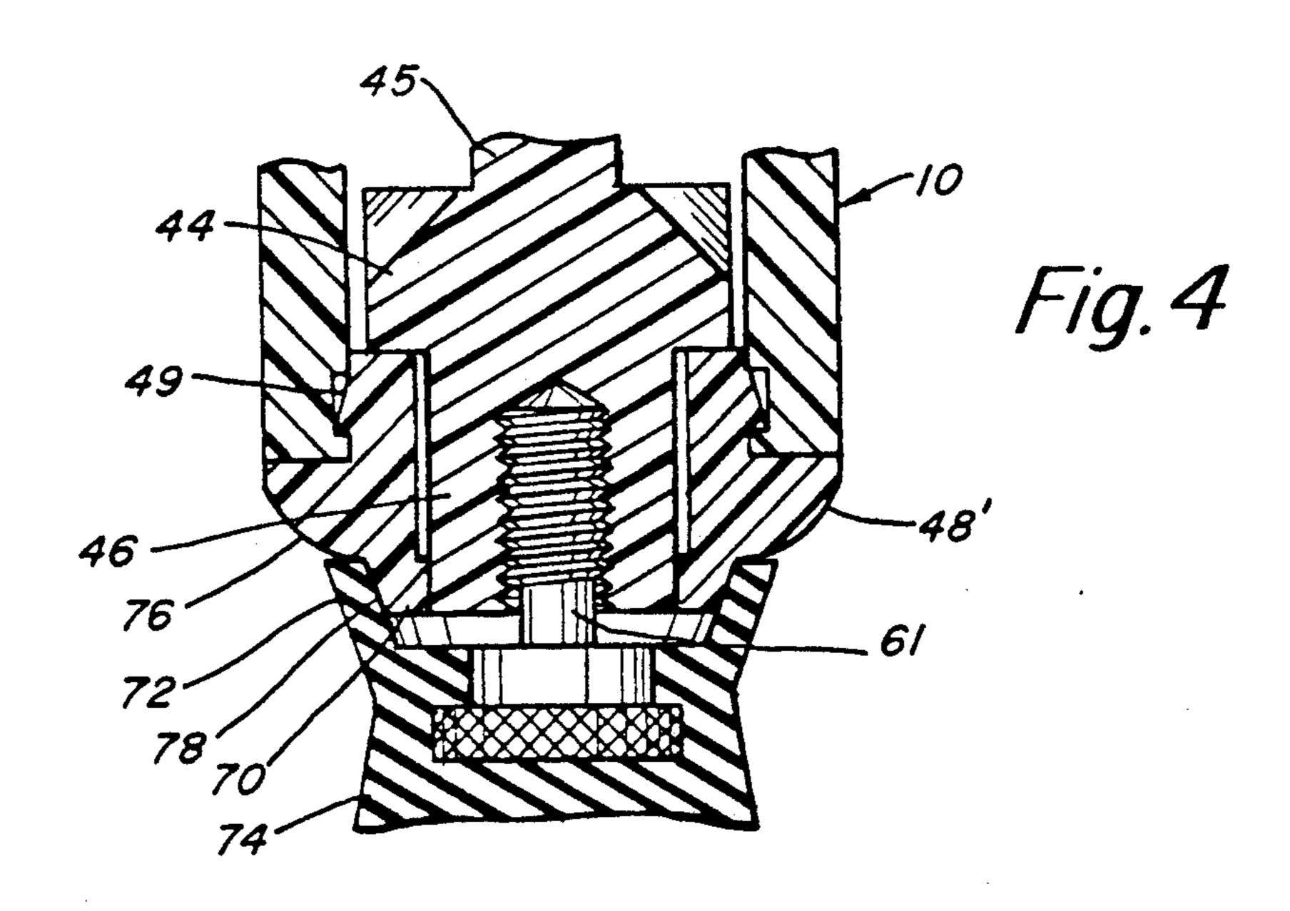
FIG. 4 is a cross-sectional view similar to FIG. 3, but illustrating a modified arrangement of the present invention.
