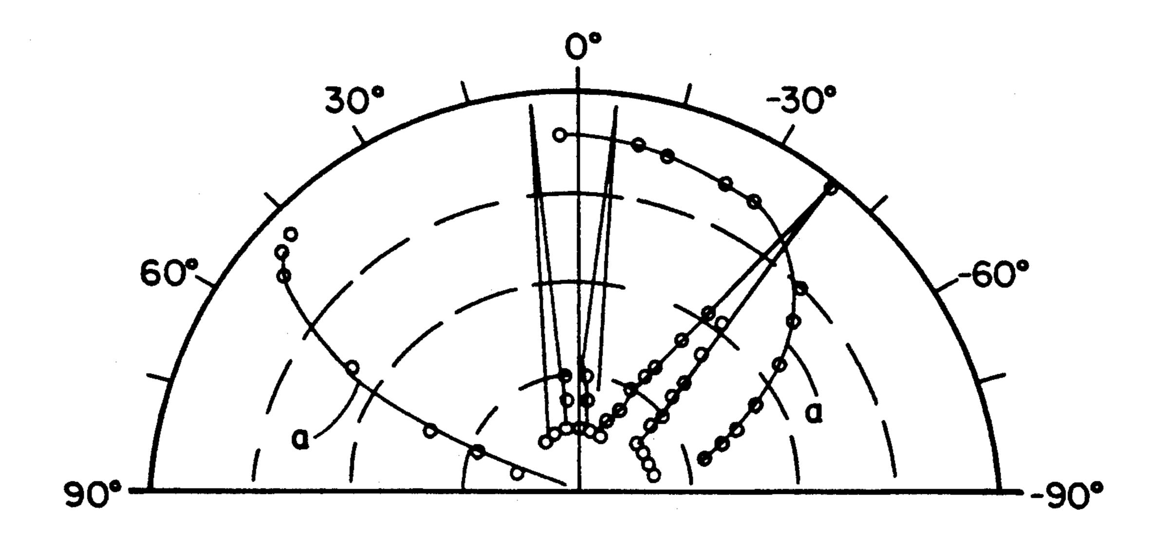
FIG.3 ANGULAR DISTRIBUTION OF THE ENHANCED TM-POLARIZED FLUORESCENCE AT THE WAVE-LENGTH 585 nm FROM A CORRUGATED STRUCTURE, AS IN FIGURE 1. 0° MARKS THE NORMAL TO THE SAMPLE SURFACE.
