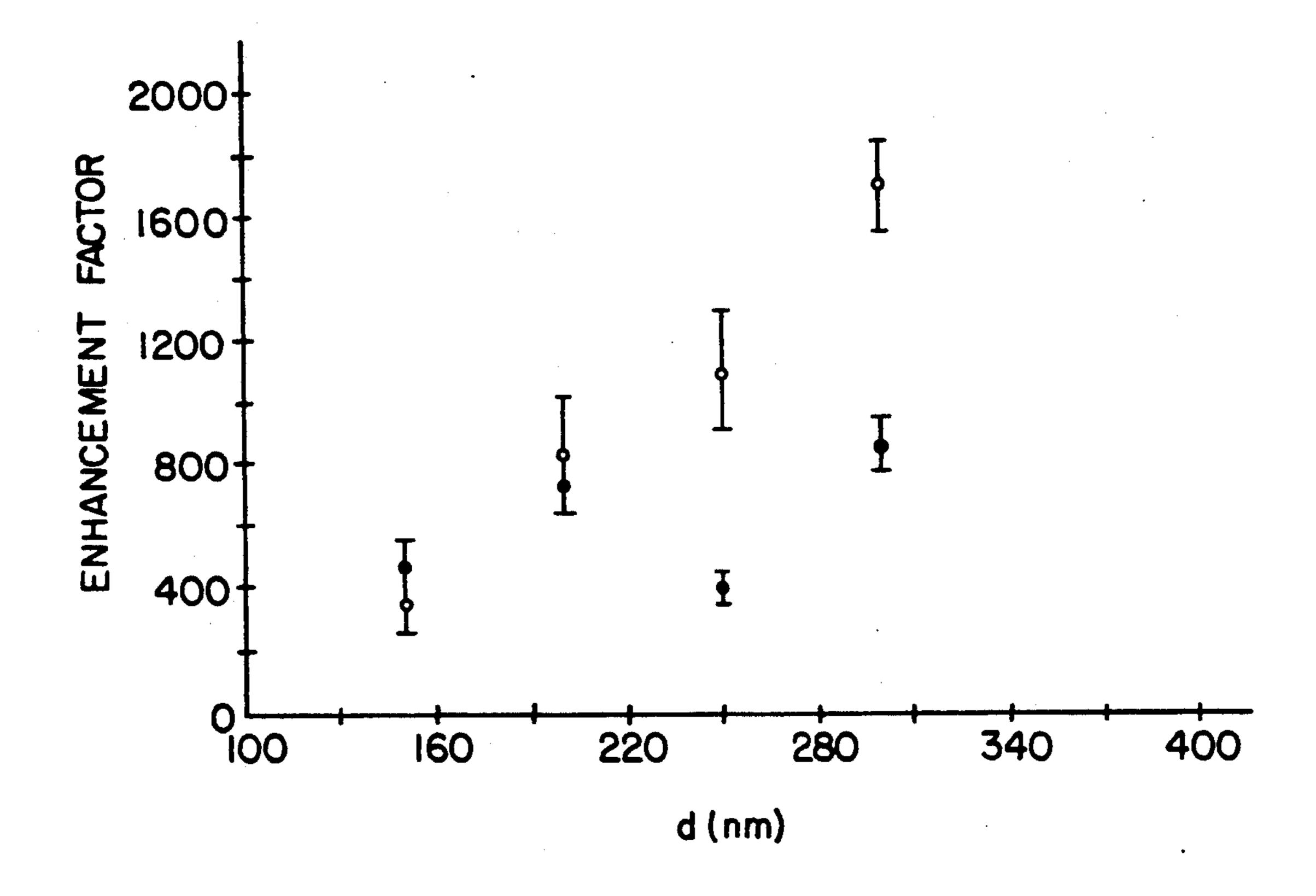
FIG.5 ENHANCEMENT FACTORS VS. WAVEGUIDE THICKNESS d OF THE TE-POLARIZED RESONANT FLUORESCENT SIGNAL EMITTED BY THE TEO-MODE. THE SOLID DOTS DENOTE THE ENHANCEMENT FACTORS FOR TM-POLARIZED EXCITING LIGHT, AND THE CIRCLES DENOTE THE ENHANCEMENT FACTORS FOR TE-POLARIZED EXCITING LIGHT.
