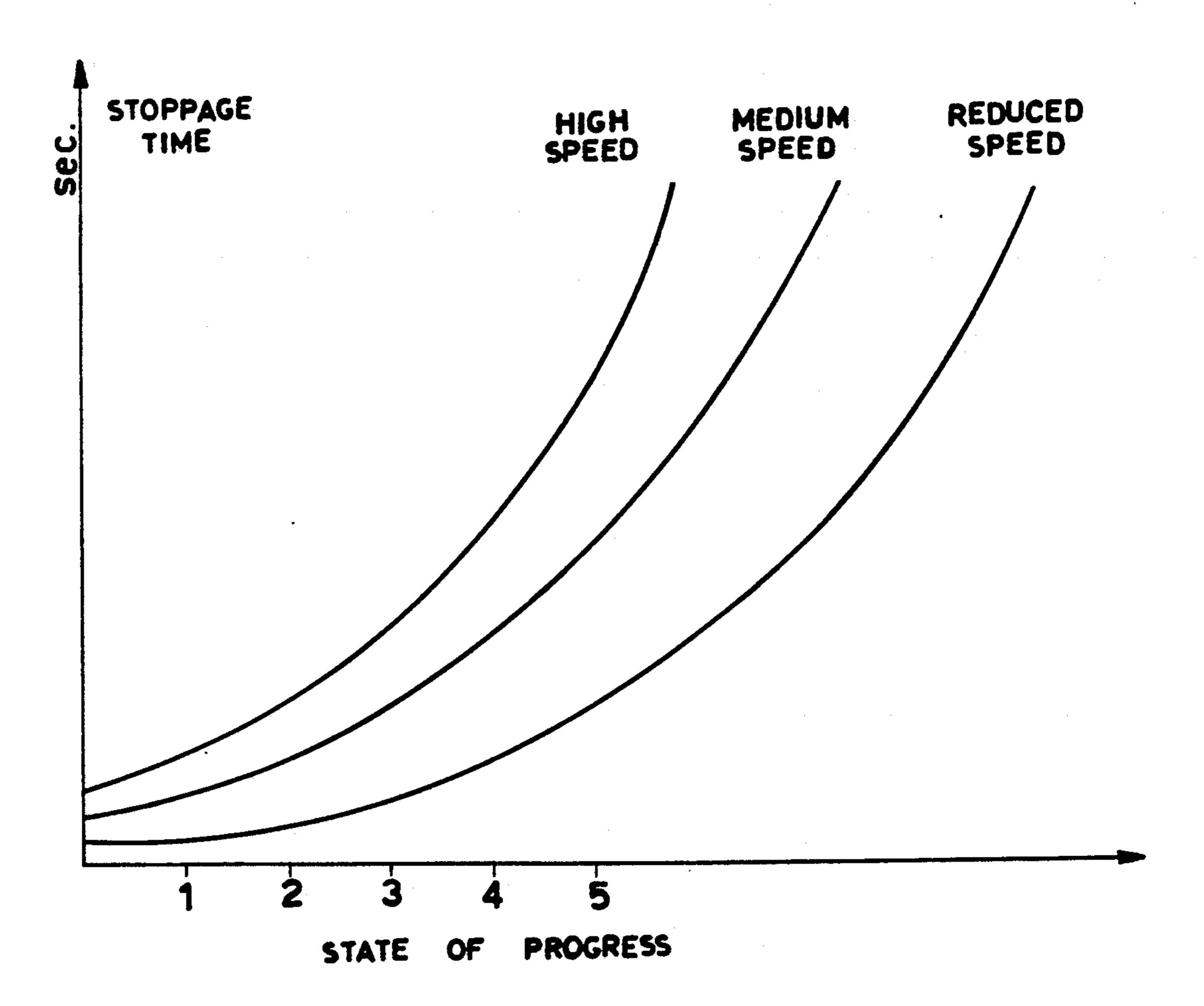
DEVELOPMENT OF THE BOBBIN STOPPAGE TIMES AS A FUNCTION OF THE WINDING SPEED
