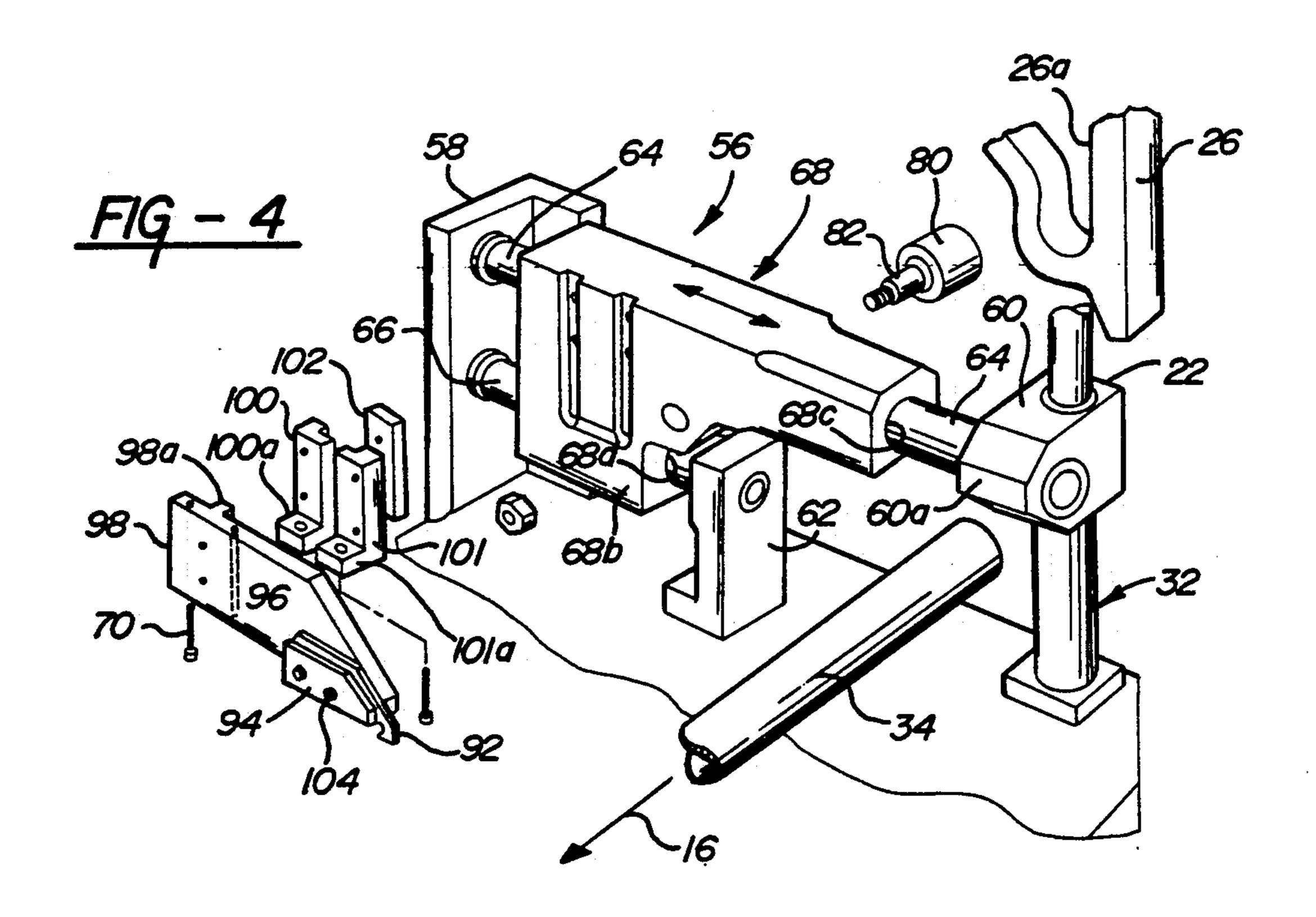
ably engage the notching blade holder at their upper ends, the head portions of the first and second screws engage the lug portions of the brackets extending outward from the cross-slide assembly.
