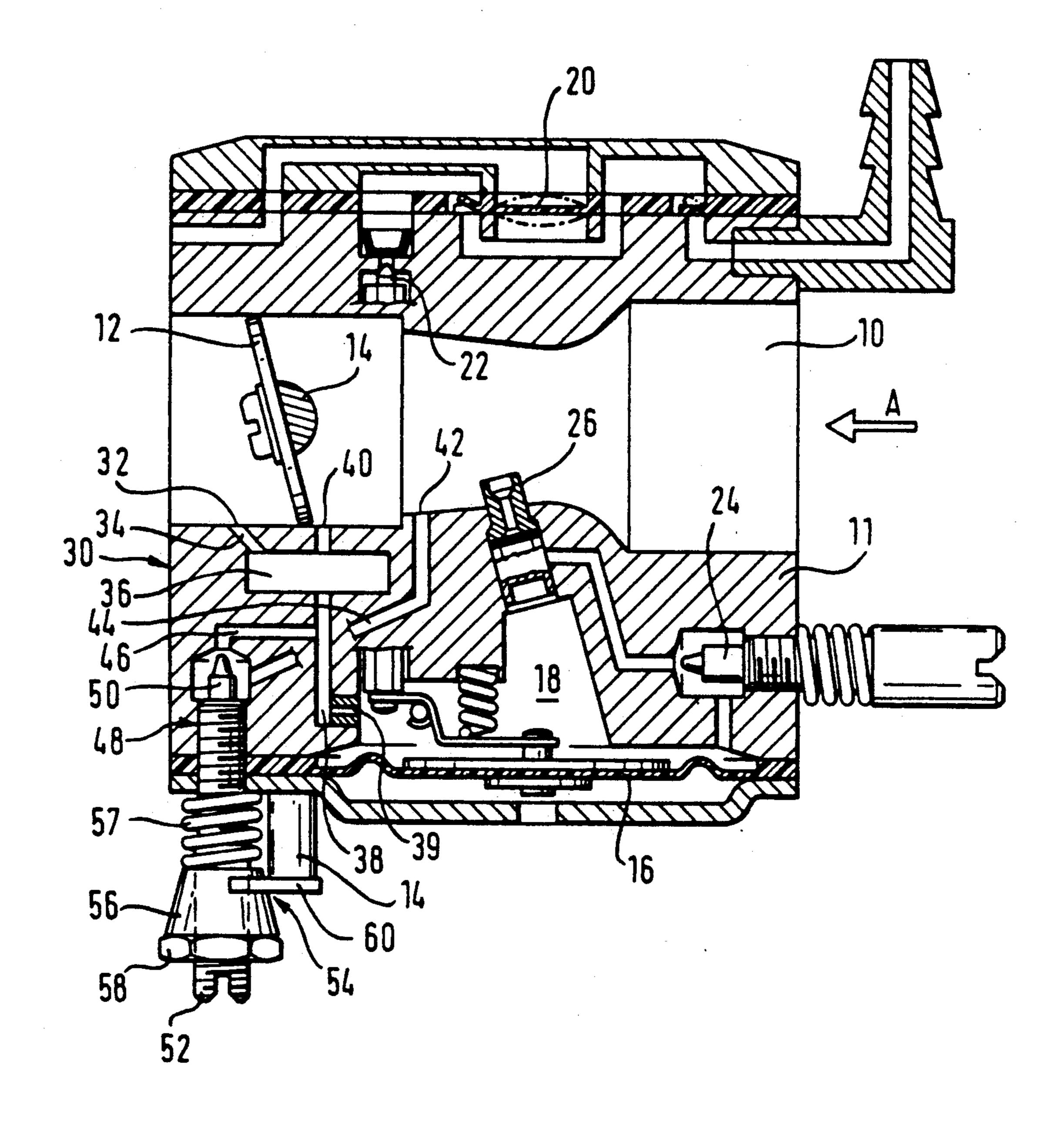
CARBURETOR INCLUDING AN IDLING ADJUSTMENT SYSTEM
