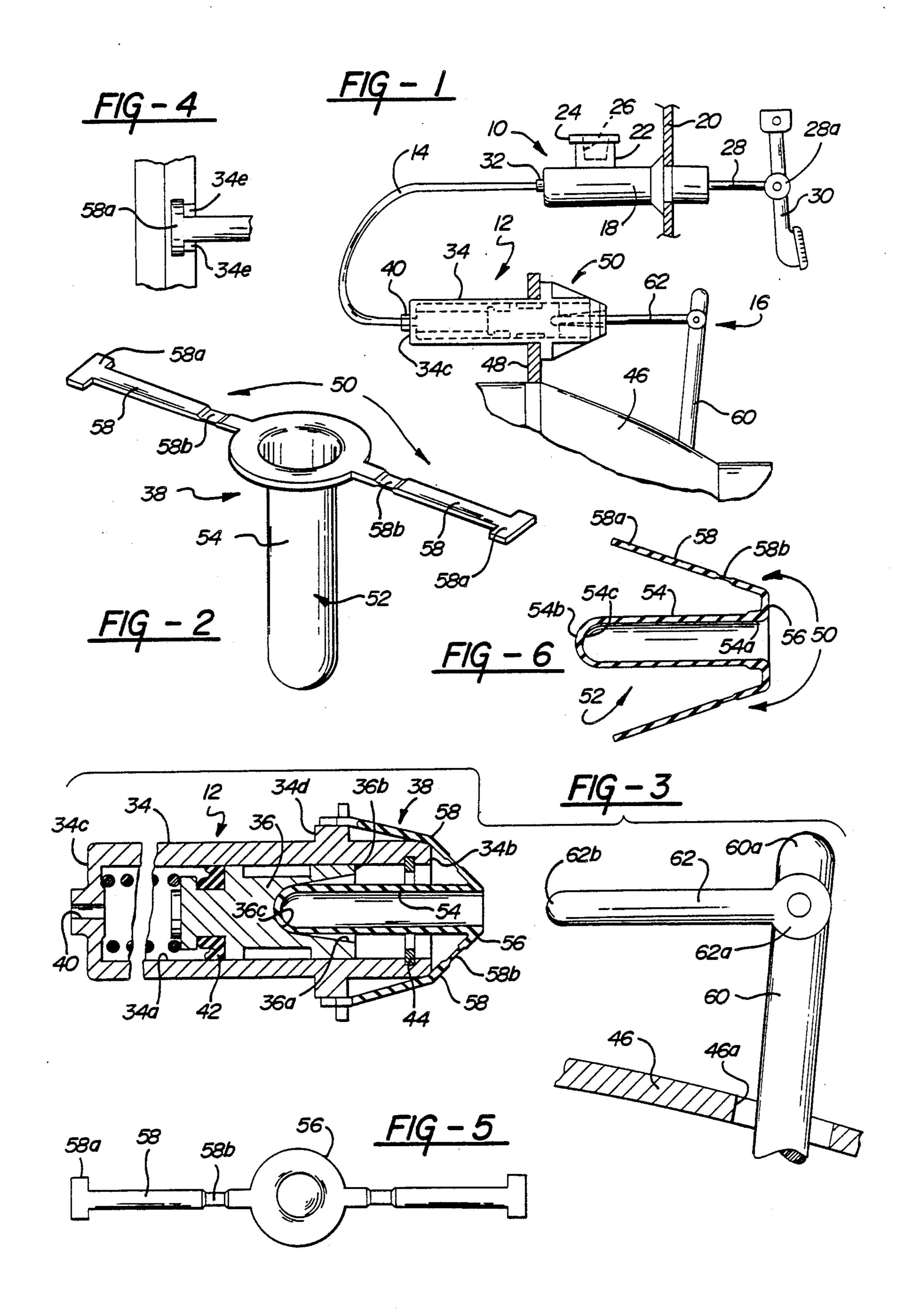
More particularly, this invention relates to a restraining strap for use with a hydraulic clutch actuator in which the slave cylinder is provided to the motor vehicle manufacturer in prefilled form but without the out-
