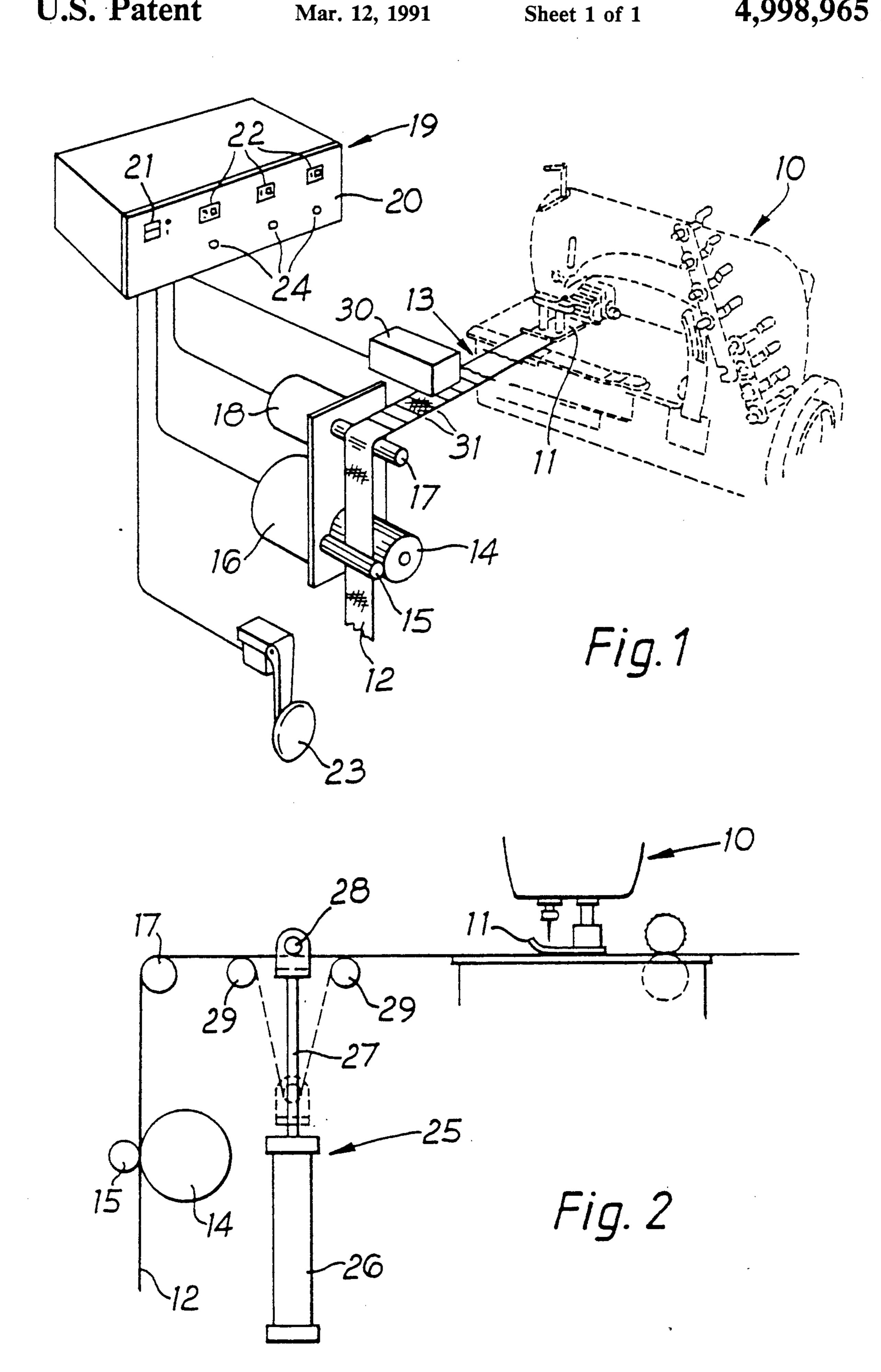
FEEDING DEVICE HAVING CONTROL MEANS, FEED ROLLERS, A PULSE GENERATOR AND A PHOTOELECTRIC DEVICE FOR DIRECTLY MEASURING RATE OF FEED OF AN ELASTIC STRIP HAVING MARKS THEREON FOR A SEWING MACHINE
