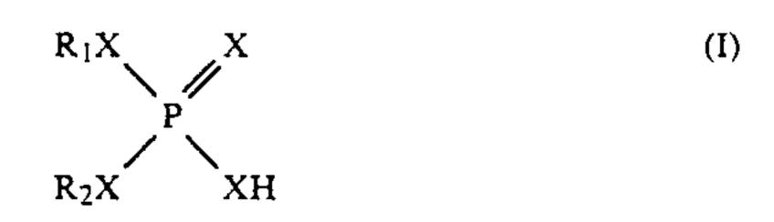
wherein R<sub>1</sub> and R<sub>2</sub> are each independently hydrocarbyl groups of from 1 to about 30 carbon atoms and X is oxygen or sulfur, with the proviso that one X is sulfur comprising reacting
